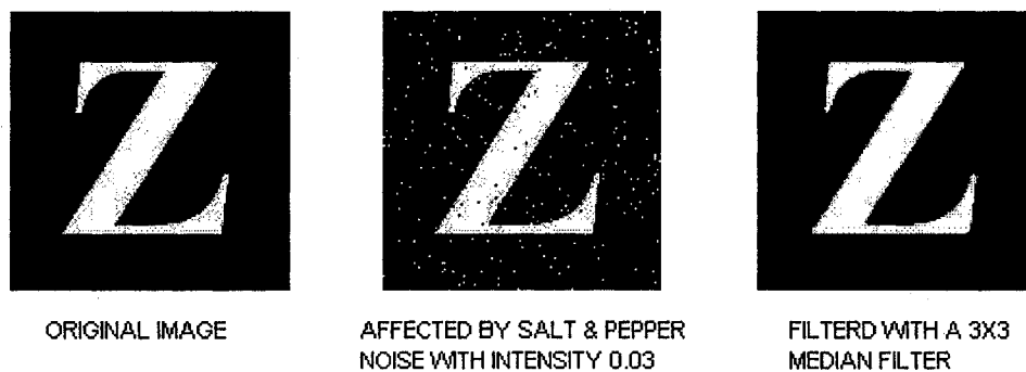
Figure 5.6: The filtering result of a 3×3 median filter on a salt and pepper affected image.
