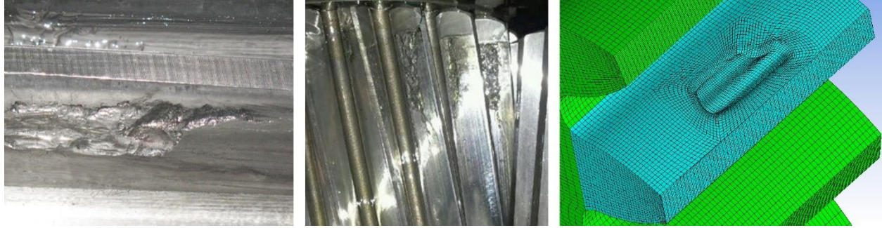
(a) Practical tooth spall (b) Practical tooth spall [148] (c) Finite element model of spall
