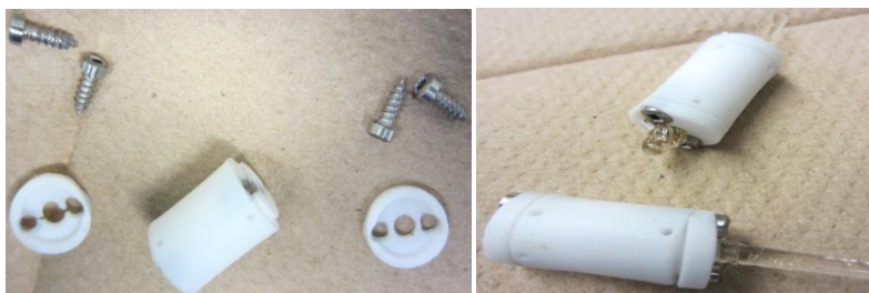
Fig 3. 1 Teflon molds (left), Vacuum dried PLGA channels within Teflon molds prior to CO 2 foaming process (right)
