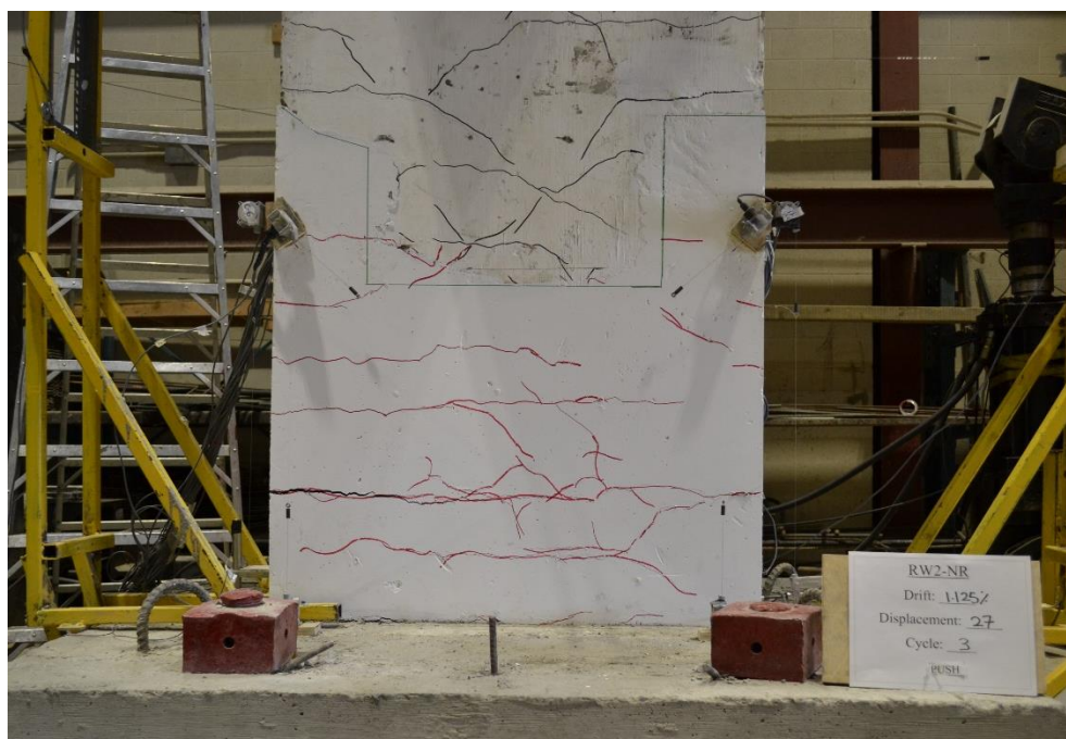
Figure A.2.4: Crack Pattern of Wall RW2-NR at 1.125% Drift (27 mm Displacement)
