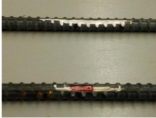
Figure 3.31: Strain Gauge Preparation on 10M bar
