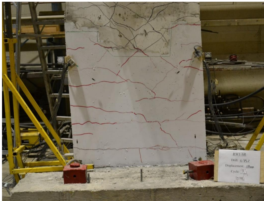
Figure A.1.5: Crack Pattern of Wall RW1-SR at 0.75% Drift (18 mm Displacement)
