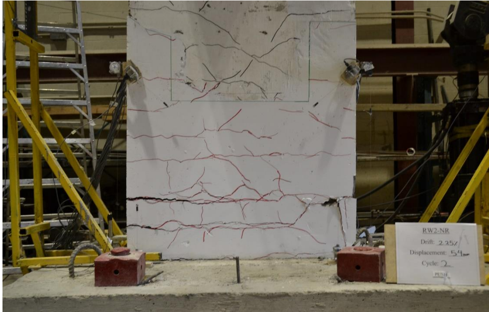
Figure A.2.7: Crack Pattern of Wall RW2-NR at 2.25% Drift (54 mm Displacement)
