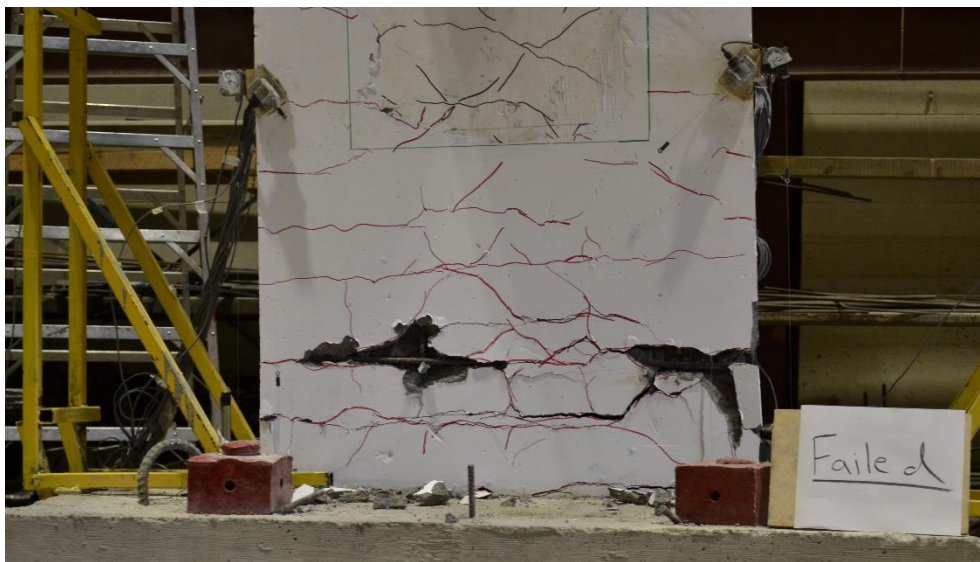
Figure A.2.142: Crack Pattern of Wall RW2-NR at Failure
