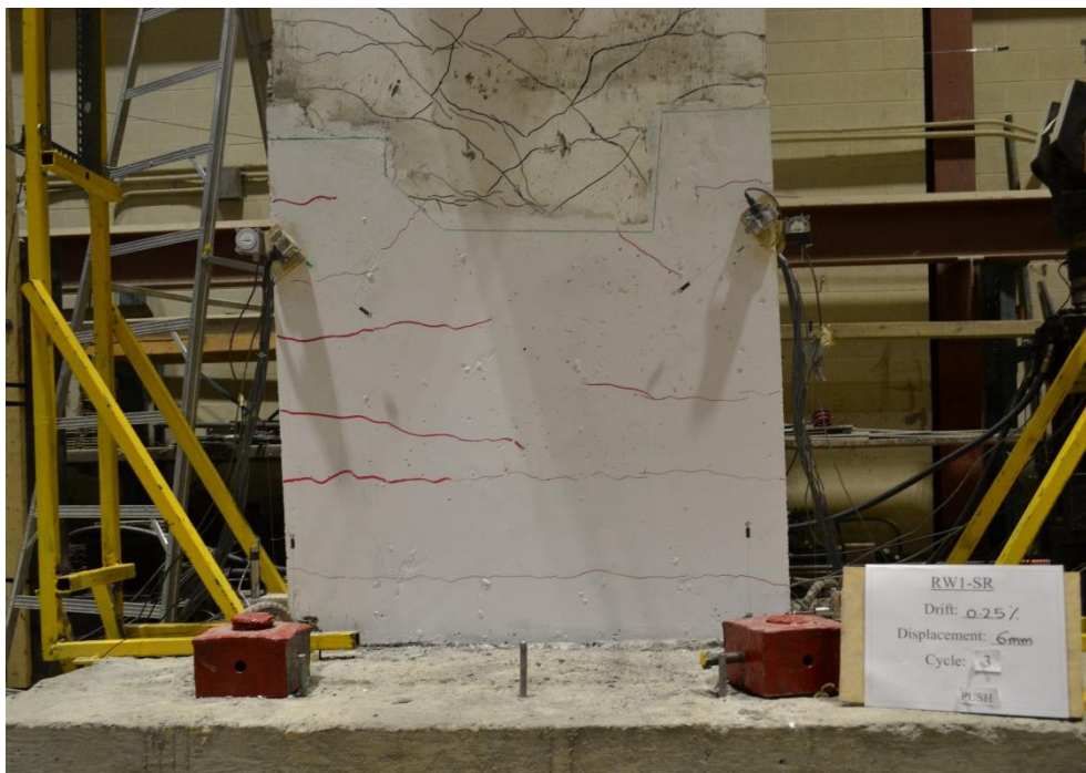
Figure A.1.3: Crack Pattern of Wall RW1-SR at 0.25% Drift (6 mm Displacement)
