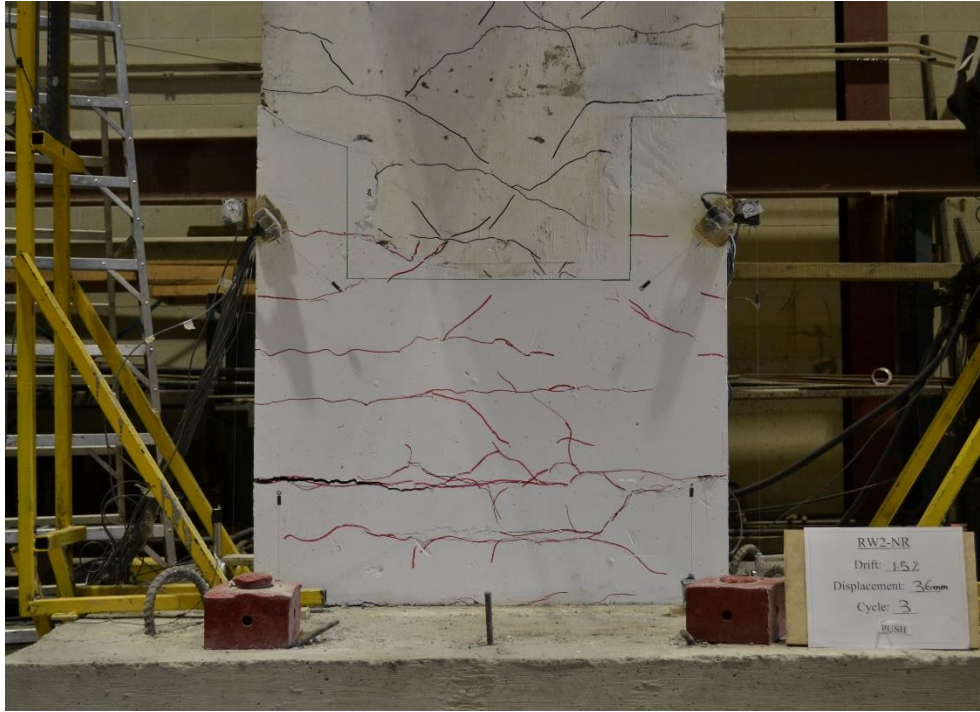
Figure A.2.5: Crack Pattern of Wall RW2-NR at 1.5% Drift (36 mm Displacement)
