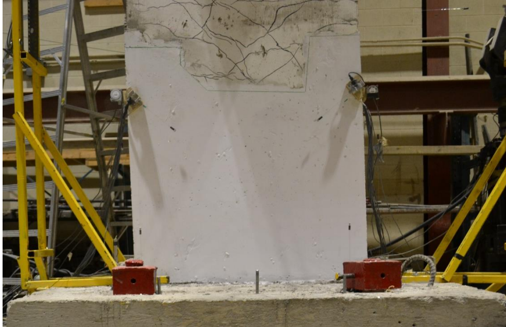
Figure A.1.1: State of Wall RW1-SR Before Testing
