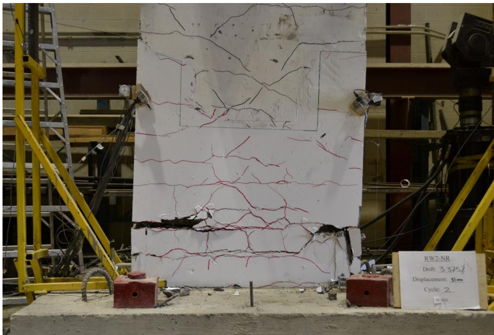
Figure A.2.10: Crack Pattern of Wall RW2-NR at 3.375% Drift (81 mm Displacement)
