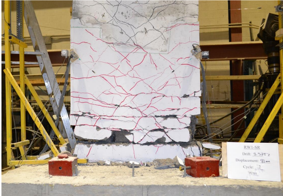
A.1.12: Crack Pattern of Wall RW1-SR at 3.375% Drift (81 mm Displacement)
