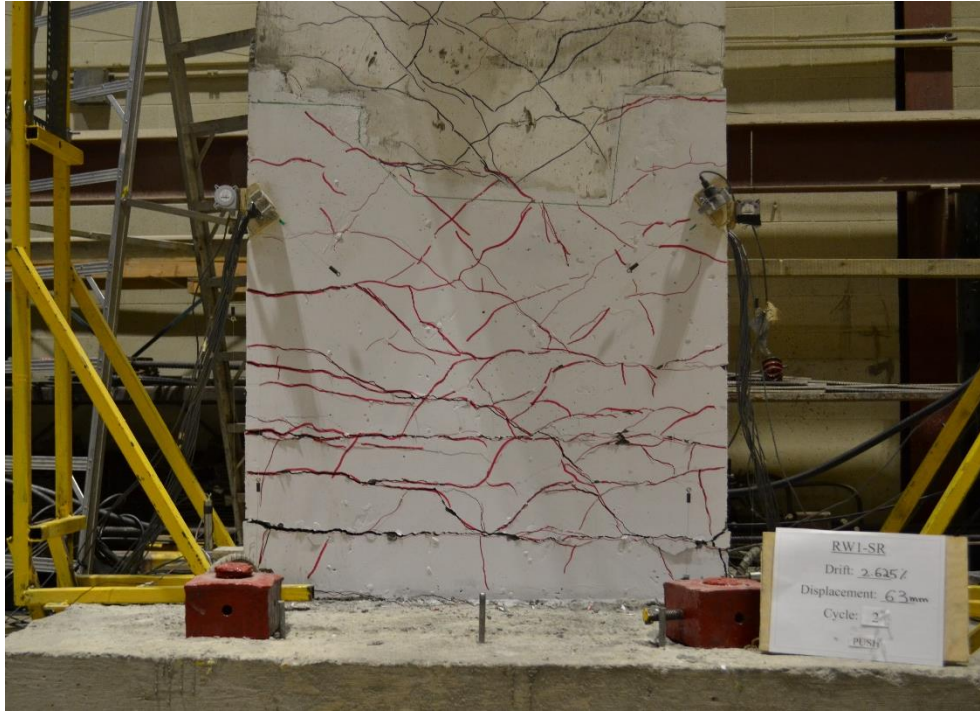
Figure A.1.10: Crack Pattern of Wall RW1-SR at 2.625% Drift (63 mm Displacement)
