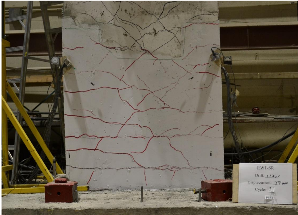
Figure A.1.6: Crack Pattern of Wall RW1-SR at 1.125% Drift (27 mm Displacement)
