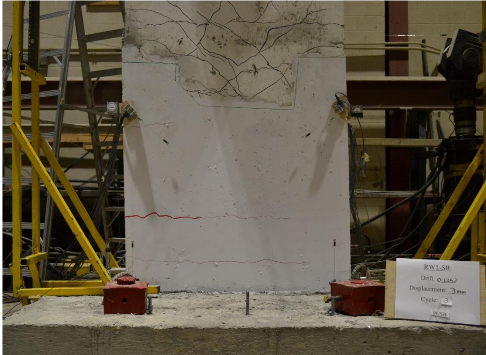
Figure A.1.2: Crack Pattern of Wall RW1-SR at 0.125% Drift (3 mm Displacement)
