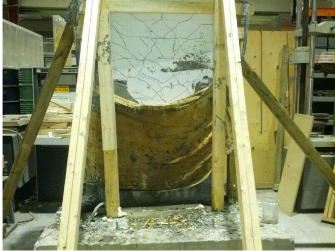
Figure 3.23: Curing of Repaired Shear Walls
