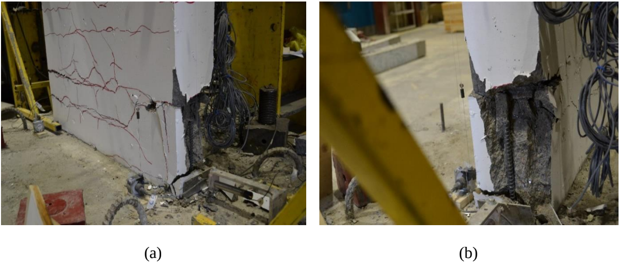
Figure 4.6: Spalled Concrete in RW2-NR at Drift Level of 2.25%: (a) Front View; and (b) Side View
