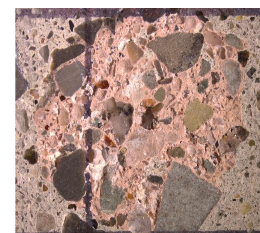
Residual mortar was easily distinguished from new mortar due to the difference of hue and texture
