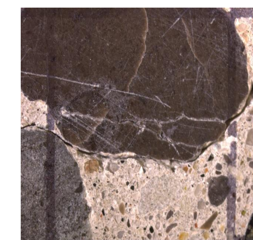
Closed crack, crack fork within the virgin aggregate and another crack propagating through the ITZ between the aggregate and the new mortar
