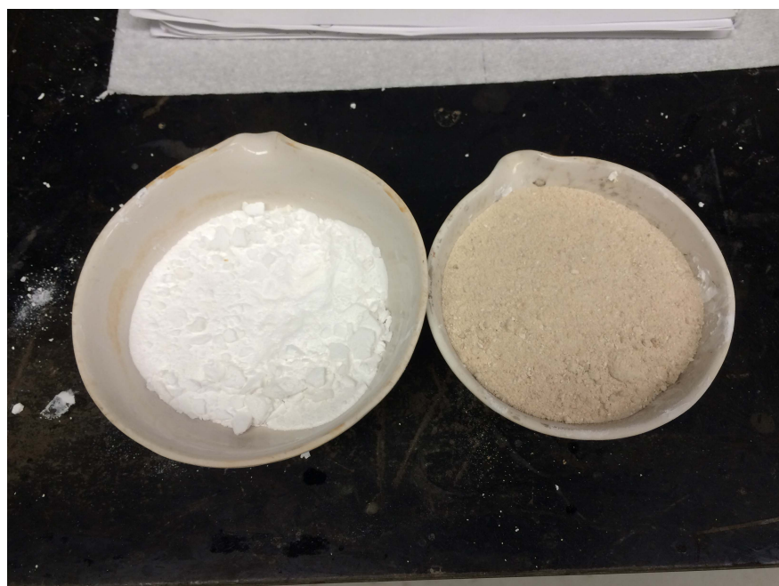
Fig. 3. 4 Dry struvite generated from synthetic solution (left) and landfill leachate (right)
