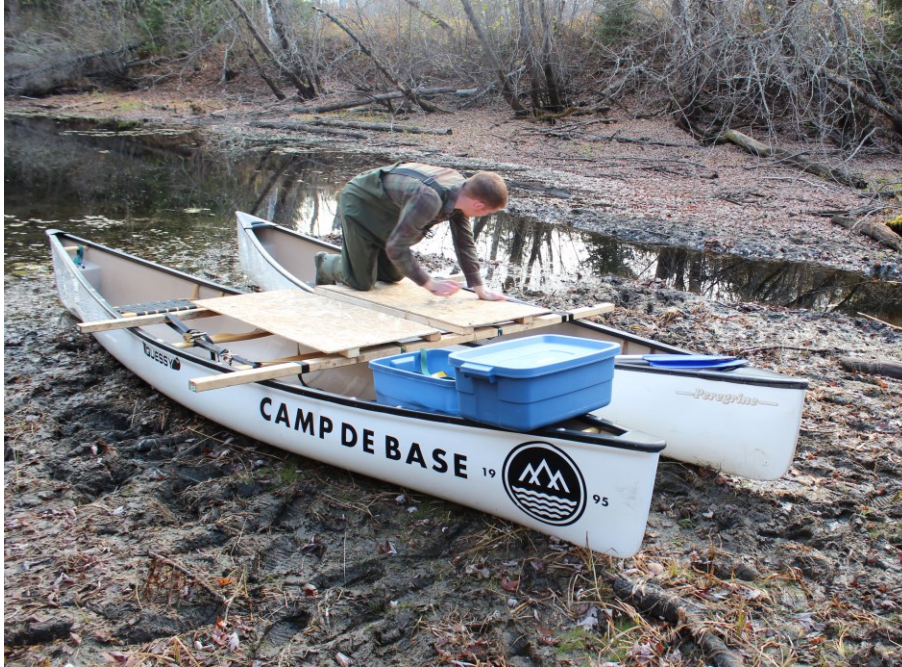
Figure 3.2.1 Coring platform built over two canoes in the field on October 16th 2012 (F. Oliva)
