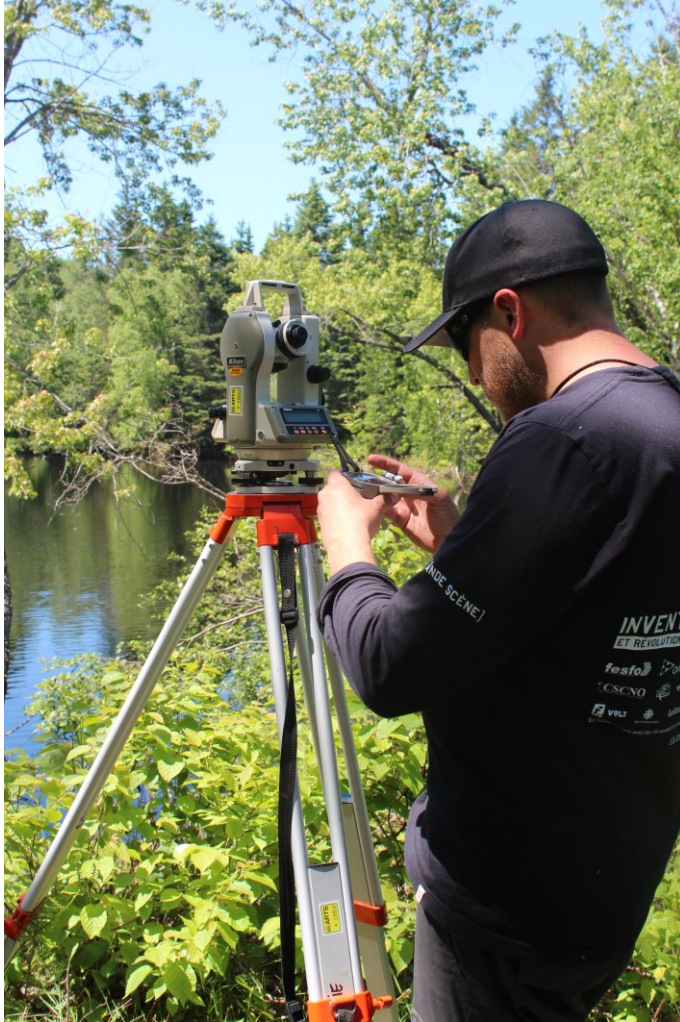
Figure 3.2.4 Nikon digital theodolite being used in the field on June 14th 2013. (K.Lafontaine-Boyer)
