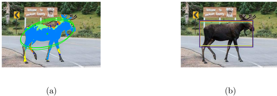
Figure 4.11: Overlapping MSER regions. (a) Six overlapping MSER regions fitted with ellipses. (b) The fitted bounding rectangles to the overlapping MSER.
