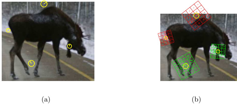
Figure 2.9: SIFT feature and descriptor. (a) The keypoints marked with yellow circle. (b) SIFT description marked with 4 \times 4 blocks.
