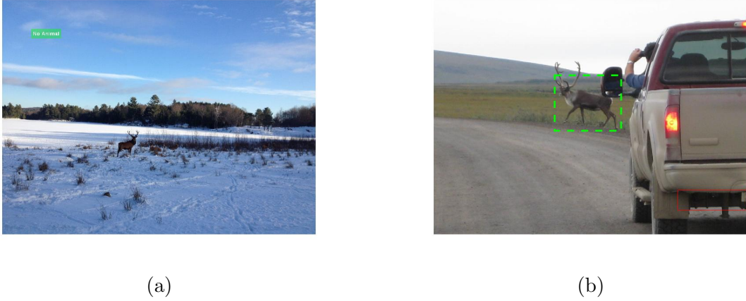
Figure 5.19: IoU is 0. (a) Animal is not found. (b) Wrong position located. The tested box is locating the back bottom part of the car.
