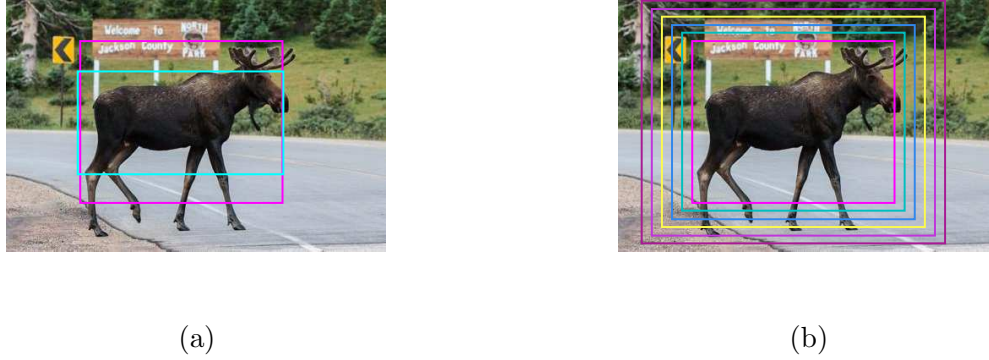
Figure 4.14: Modification and enlarging of MSER box. (a) Extend the shorter by fixed rate. (b) MSER box is enlarged along both width and height by 1.1 to 1.5, stride=0.1.
