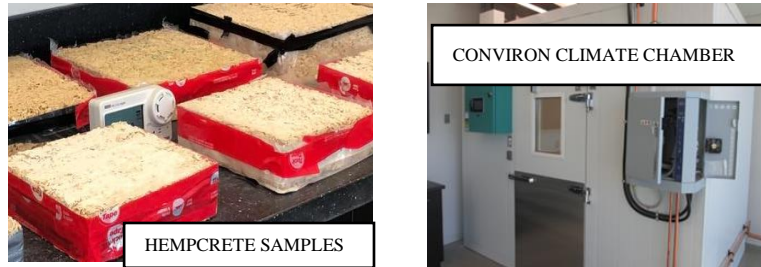
Figure 3.4. Hempcrete samples for testing and chamber.
