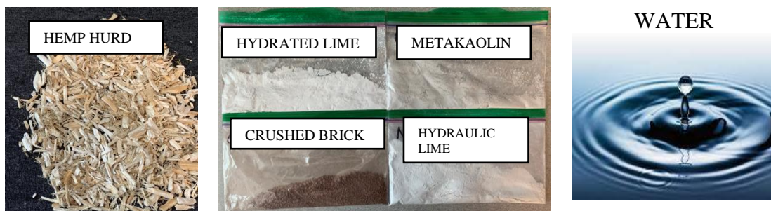
Figure 3.2. Hempcrete ingredients of different mix designs.
