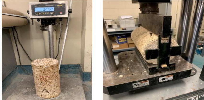
Figure 3.6. Hempcrete sample and tensile test measurement using UTS.
