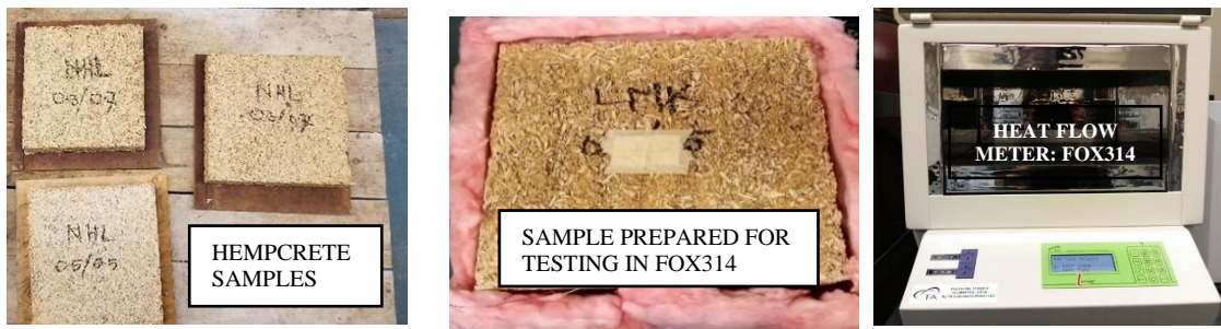
Figure 3.3. Hempcrete samples and heat flow meter.
