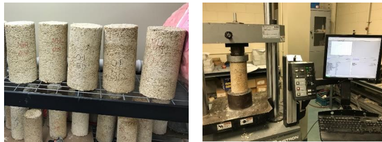
Figure 3.5. Hempcrete samples prepared for testing and universal testing system (UTS).
