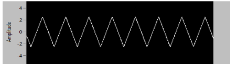
Figure 2.8 Triangular signal used as input for the bimorph slider, typically here 5V peak-to-peak amplitude at 0.05Hz
