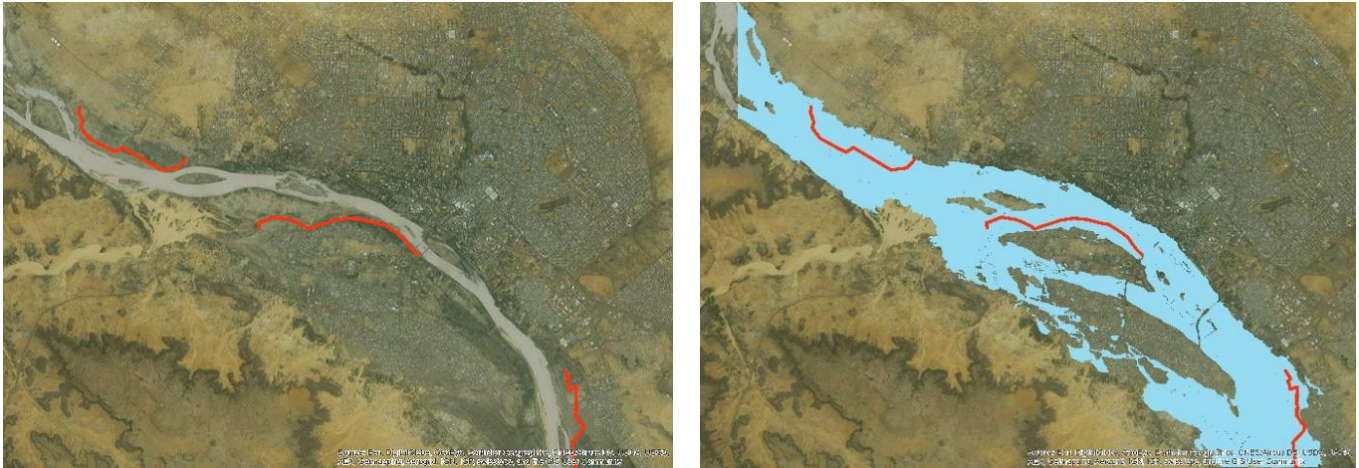
Figure 2.4. Location of flood protection dikes (red lines) in Niamey, and extent of the 2012 flood (in blue).
