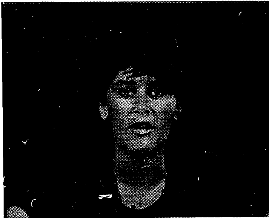
Figure 4.13: Reconstructed frame number 64 of the Miss America sequence using VC-FAVQ at 0.25 bpp.
