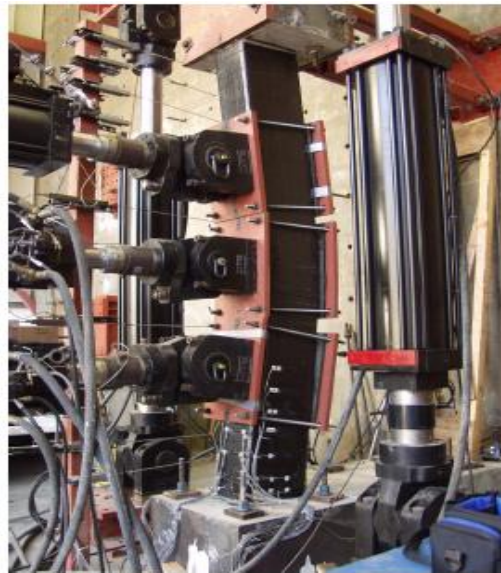
Figure 2.5: Full scale CFRP RC column tested by lateral loading system
