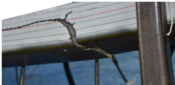
Figure 4.62. Damage to Column S8 at maximum load
