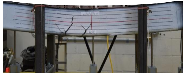
Figure 4.80. Damage on side face of Column S9 at maximum load
