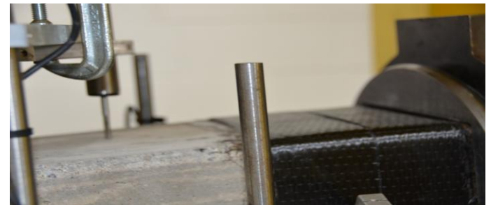
Figure 4.15. Damage to Column S6 near the hinge support
