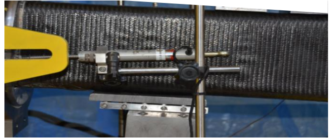
Figure 4.59. Damage to Column S8 near the roller support
