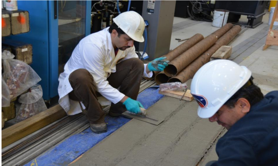
Figure 3. 19. Using of curbing trowel to smooth the top edges of all column specimens
