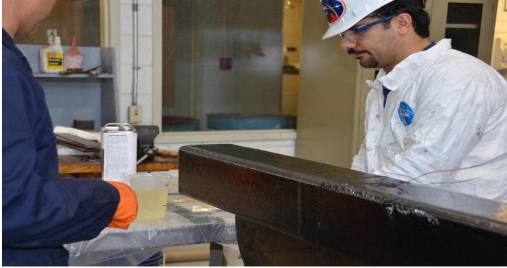
Figure 3. 21. Wrapping the stripped ends of a specimen
