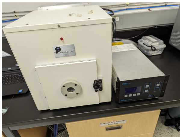
Figure 3.3: Plasma Etch PE-50 cleaner used for the oxygen plasma treatment of a silver pellet.
