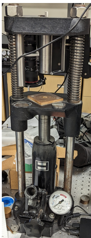
Figure 3.2: Press used to prepare the silver pellets.
