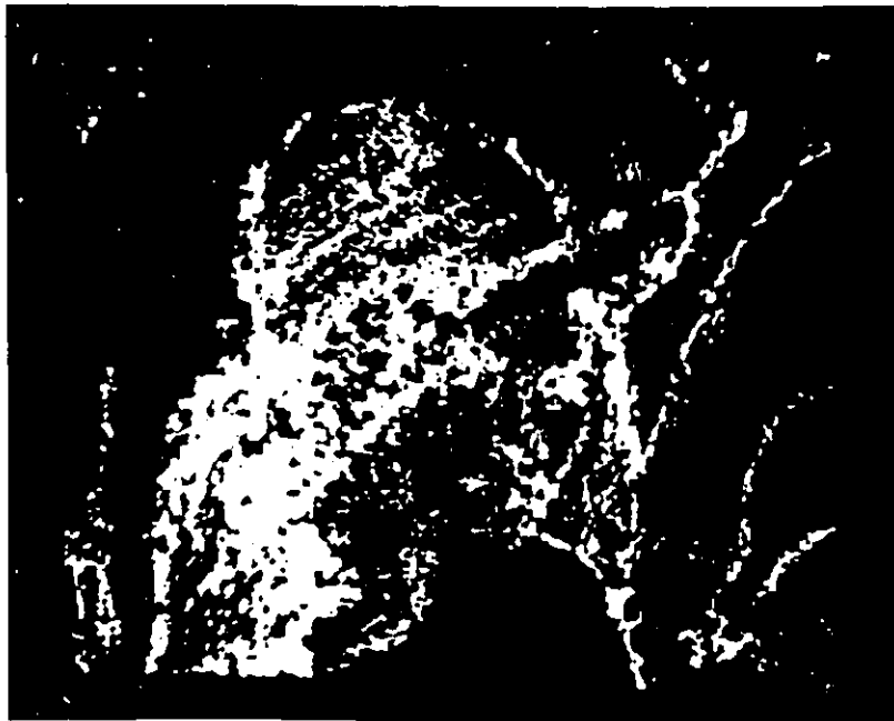
Fig. 5.13 The error Face (Lena) image using VQRUC-1 with 16-D vectors at a bit rate of 1.42 bits/pixel
