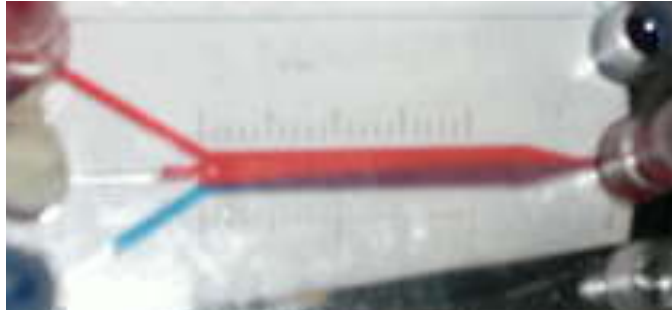
Figure A.28: Experimental set up for the experiment with the different flow rate for both branches. The two fluid flow in the 3mm width channel can also clearly be visualized.
