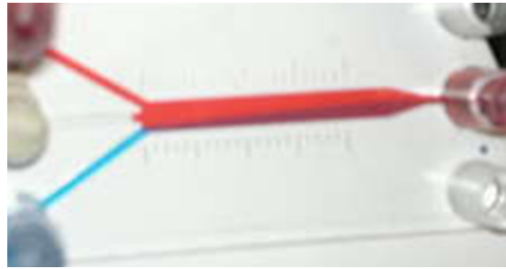
Figure A.25: Experimental set up for the experiment with the same flow rate for both branches. The two fluid flow in the 3mm width channel can clearly be visualized.
