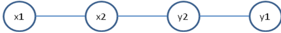
Figure 8: Problems in on-demand BSF algorithms I. This scenario shows one of the problems that on-demand BSF algorithms need to address. The circles represent the nodes; x_1 , x_2 , y_2 and y_1 , while the lines represent the links between the nodes. If both y_1 and x_1 wanted to contact each other at the same time, then y_2 and x_2 may need to alternate between the INQUIRY and INQUIRY SCAN states for them to discover each other.
