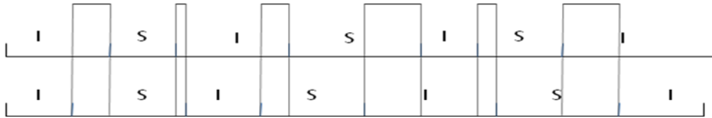
Figure 6: Illustration of the device discovery technique of Salonidis et al. [36]. This figure illustrates a scenario in which two nodes are executing this discovery technique. The two nodes cannot discovery with each other except if they were in opposite states. These time slots are represented with the rectangles.
