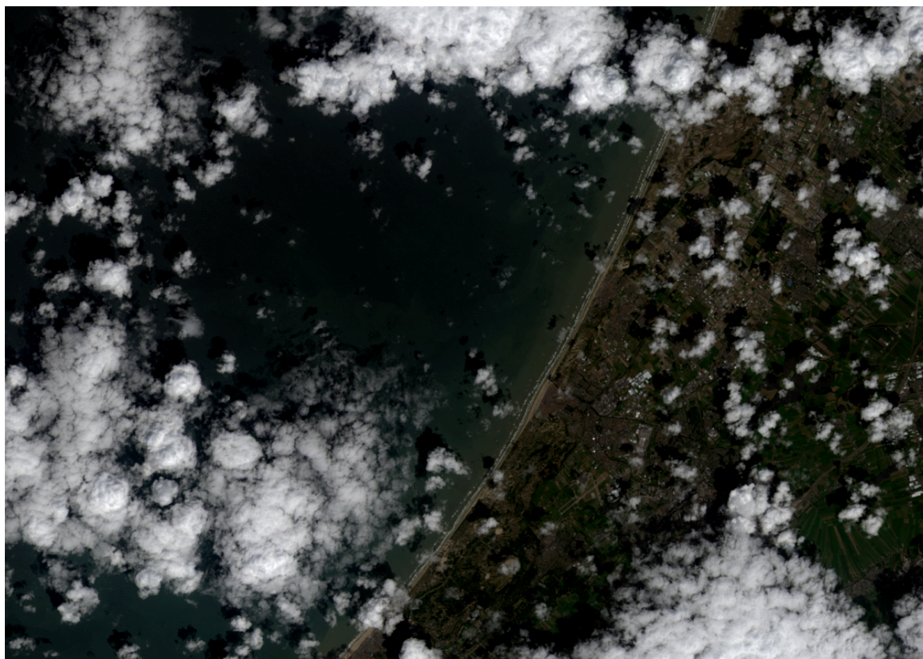
Figure 36: Linear contrast enhancement using the minimum and maximum values of the image in place of 50 and 240 in the above example. By Anders Knudby, CC BY 4.0 .
