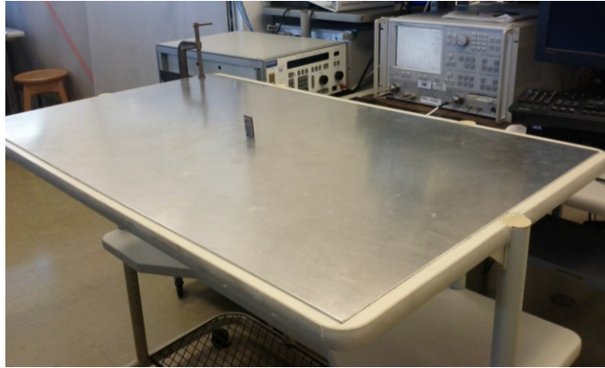
a) antenna soldered to center pin of SMA connector and is mounted on a metal plate
