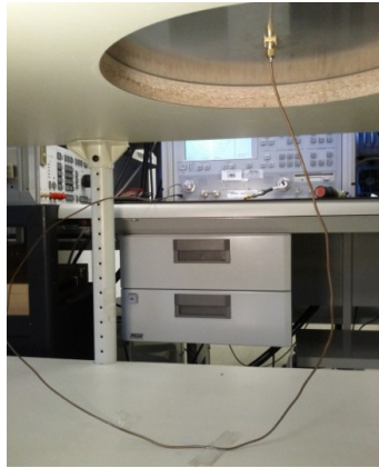
b) VNA connection to SMA connector
