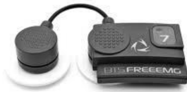
Figure 9. BTS FreeEMG wireless electrode used for recording muscle activation.
