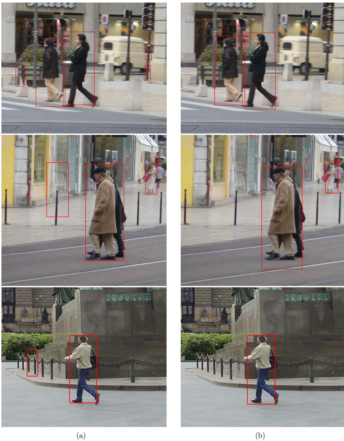
Figure 4.17: Comparison examples of the results which is pillar-like objects ( Type III ). (a) the HOG linear SVM model; (b) our proposed model.
