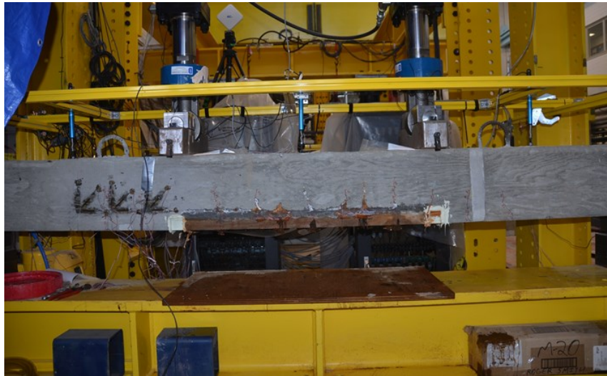
(a) at the end of the corrosion phase
