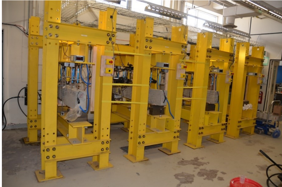
Figure 3.3: Testing frames for small-scale RC beams
