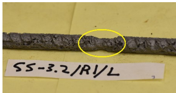
(c) Localized crack corrosion
