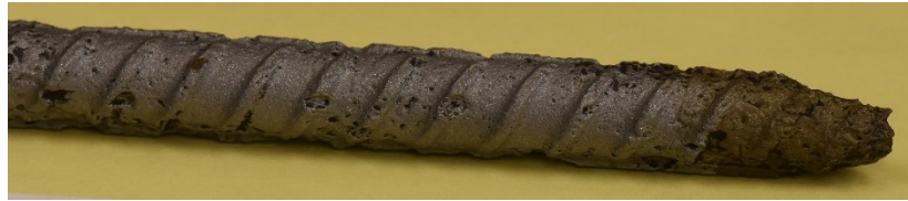
Figure 3.8: Corrosion pattern on the longitudinal steel bar facing: (a) concrete cover (b) inner core concrete
