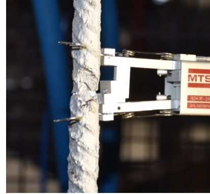
(b) Close up at the failure
