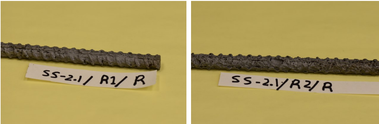
Figure A.18: Corrosion patterns on the clean surface of steel reinforcement – beam SS-2.1
