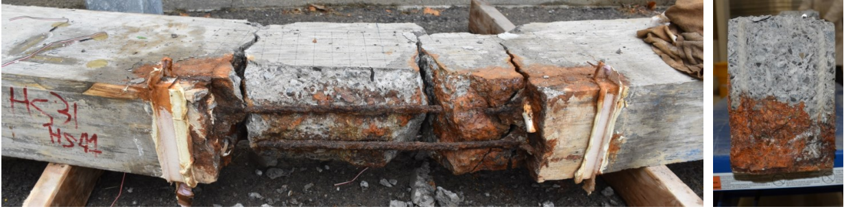
Figure 3.7: Corrosion damage: (a) across the entire length of the affected zone (b) cross-sectional
