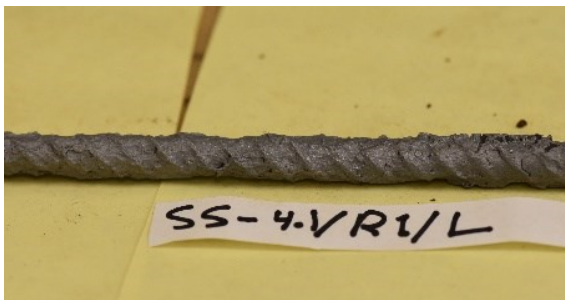
(a) Generalized corrosion
