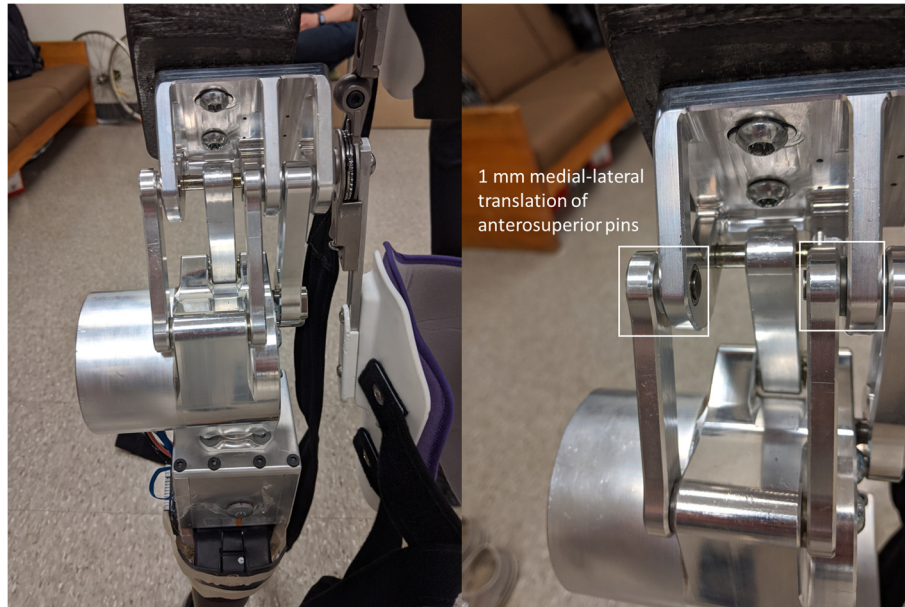
Figure 9-8: Medial-laterally translated anterosuperior pins observed after the completion of level-walking trials with three able-bodied participants.
