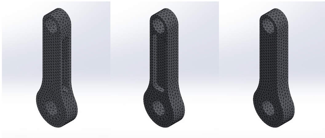
Figure 6-14: FEA meshes for drive arms 1 (left), 2 (middle), and 3 (right). Mostly uniform meshing.
