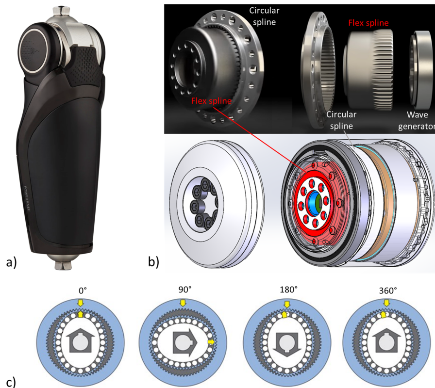
Figure 2-23: a) Össur Power Knee with a brushless DC motor at the proximal end [10], b) harmonic drive implemented in the Össur Power Knee brushless DC motor (adapted from [169]), c) harmonic drive operation (adapted from [170]).
