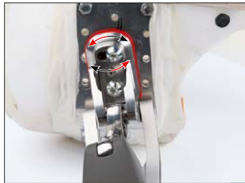
Figure 2-14: Frontal plane alignment adjustment for the Helix3D hip joint [60].
