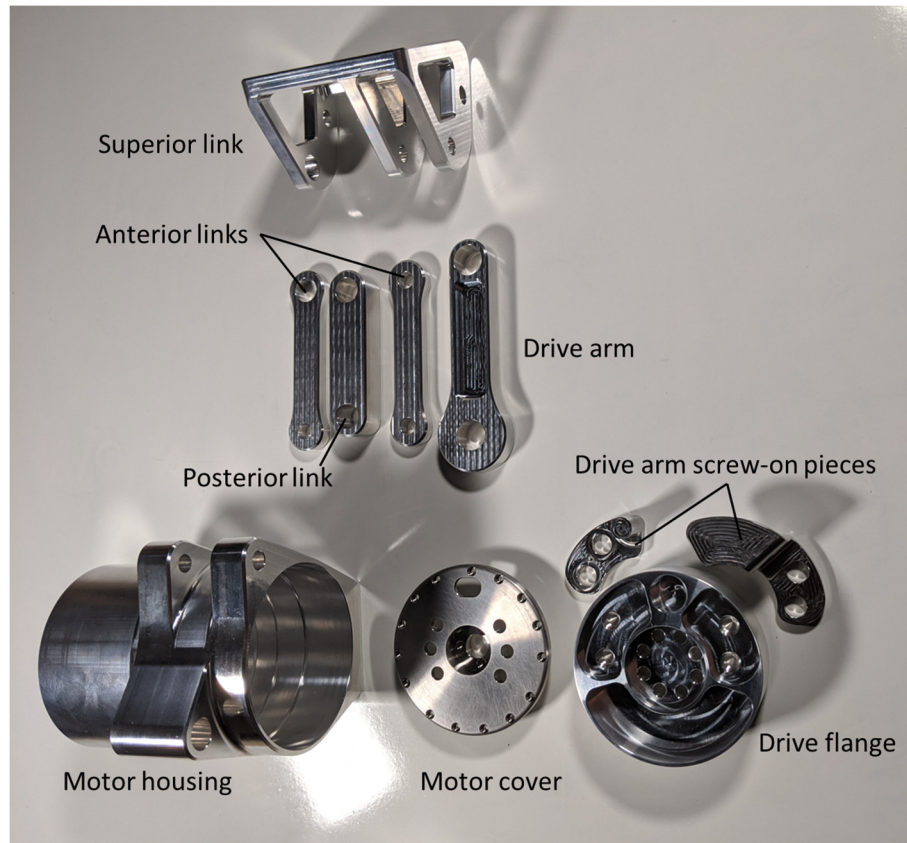
Figure 8-5: Powered hip CNC machined components. The superior link, drive arm, anterior links, posterior link, drive flange, and motor housing are made of Al 2024-T351. The drive arm screw-on pieces, and motor cover are made of 17-4 PH SS H900.
