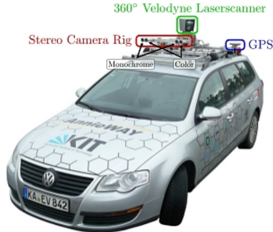
(a) Data acquisition platform
