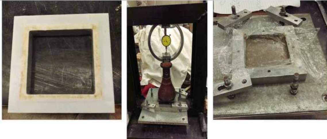
Figure 43: Shear box with Teflon layer (left); Sample being compacted in load frame with proving ring(centre); Sample after compaction (right)
