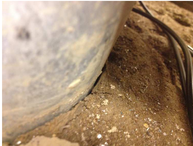
Figure 33: Soil interface separation at the surface of the sample
