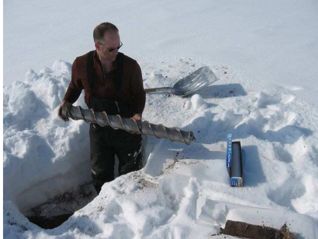
Figure 4: Removing a sample from a core barrel (SnowNet, 2009)
