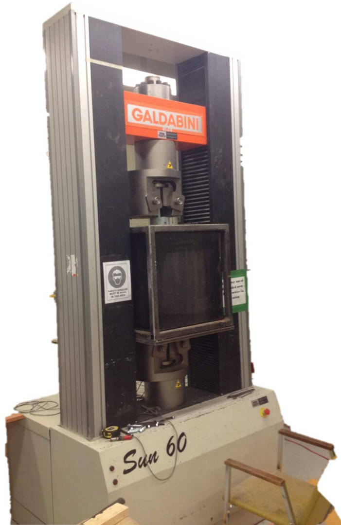
Figure 21: Galdabini Sun 60 set up with frozen soil test box
