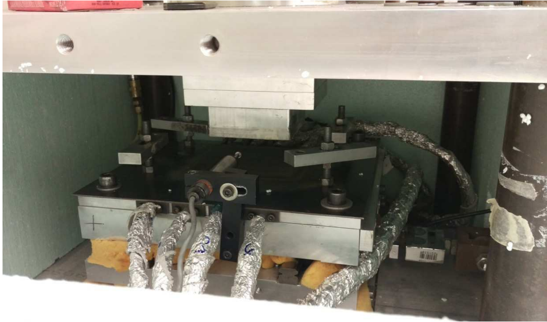
Figure 36: Interface testing table inside the insulated chamber
