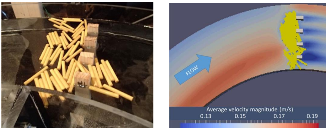
(a) Deposition and driftwood jamming (b) i-RIC simulation of debris jamming
