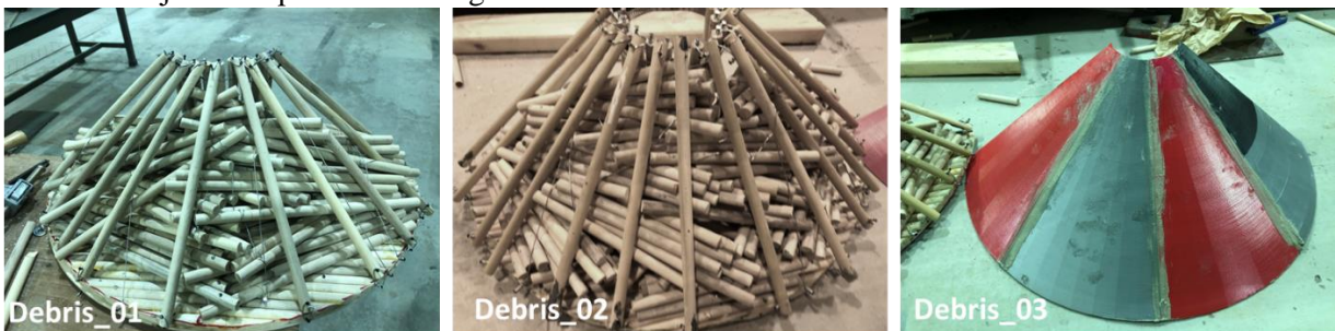
Figure 7-3 (1)Debris jam built by 30 cm length dowels (2) Debris jam built by 20 cm length dowels (3) 3D printed debris jam
