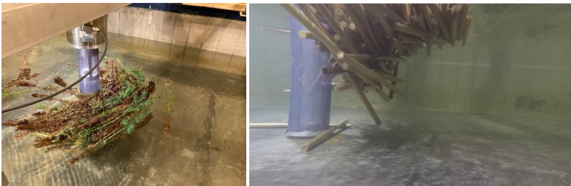
Figure 6-4 A debris jam formed by the (a) seedling trees and (b) side view for dowels.
