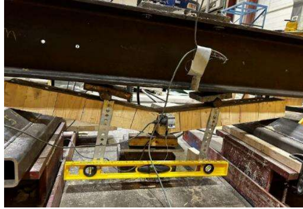
Figure 5.8: Mid-span failure observed in the beam during Specimen B01, Test 3
