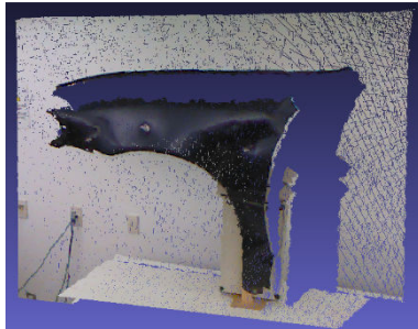
b) Raw 3D point cloud of the scene as captured by the Kinect (294664 points)
