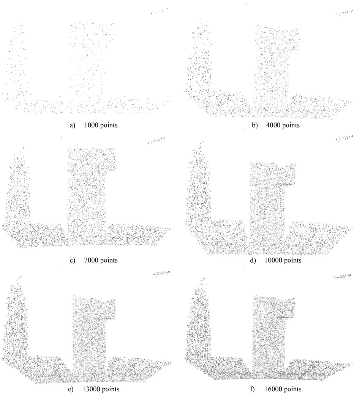
Figure 5.30 - Scene 1: probabilistic occupancy grid model (for P(\text{Occ}) > 0.5 ) progression after different numbers of points are acquired using the probabilistic occupancy grid improvement based selection process
