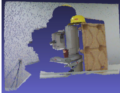
b) Raw 3D point cloud of the scene as captured by the Kinect (290427 points)
