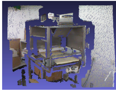
b) Raw 3D point cloud of the scene as captured by the Kinect (260103 points)
