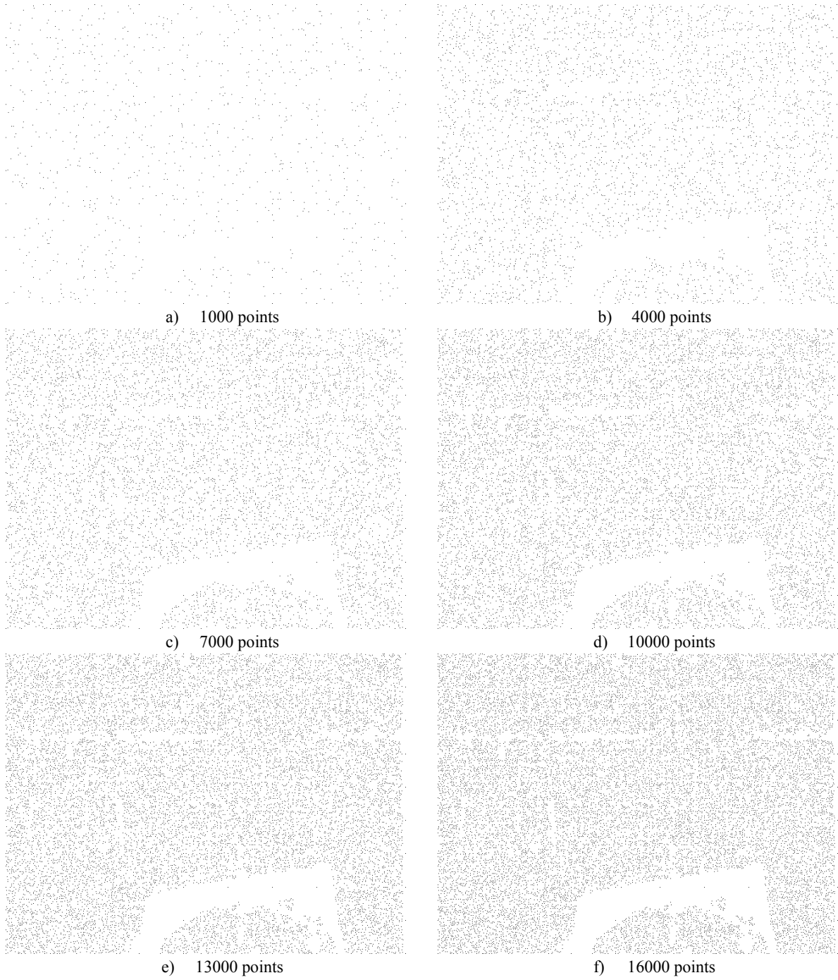
Figure 5.34 - Scene 6: point selection map progression after different numbers of points are acquired using the probabilistic occupancy grid improvement based selection process
