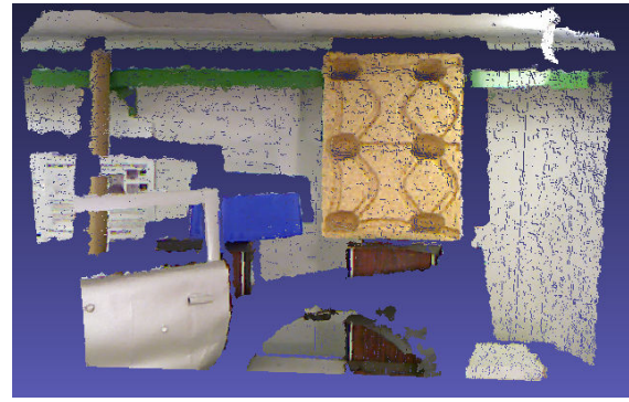
b) Raw 3D point cloud of the scene as captured by the Kinect (277753 points)
