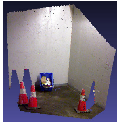
b) Raw 3D point cloud of the scene as captured by the Kinect (307200 points)
