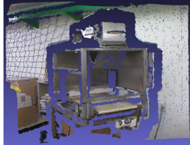
b) Raw 3D point cloud of the scene as captured by the Kinect (263302 points)
