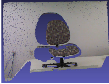
b) Raw 3D point cloud of the scene as captured by the Kinect (294237 points)
