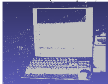
e) Raw 3D point cloud of the scene as captured by the Jupiter/Track (left side, 127441 points)
