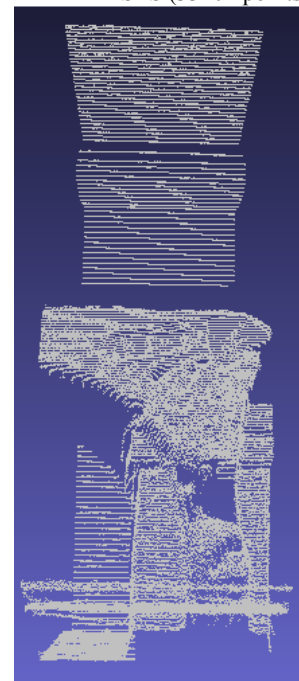
g) Raw 3D point cloud of the scene as captured by the SICK/Track (rear, 91897 points)
