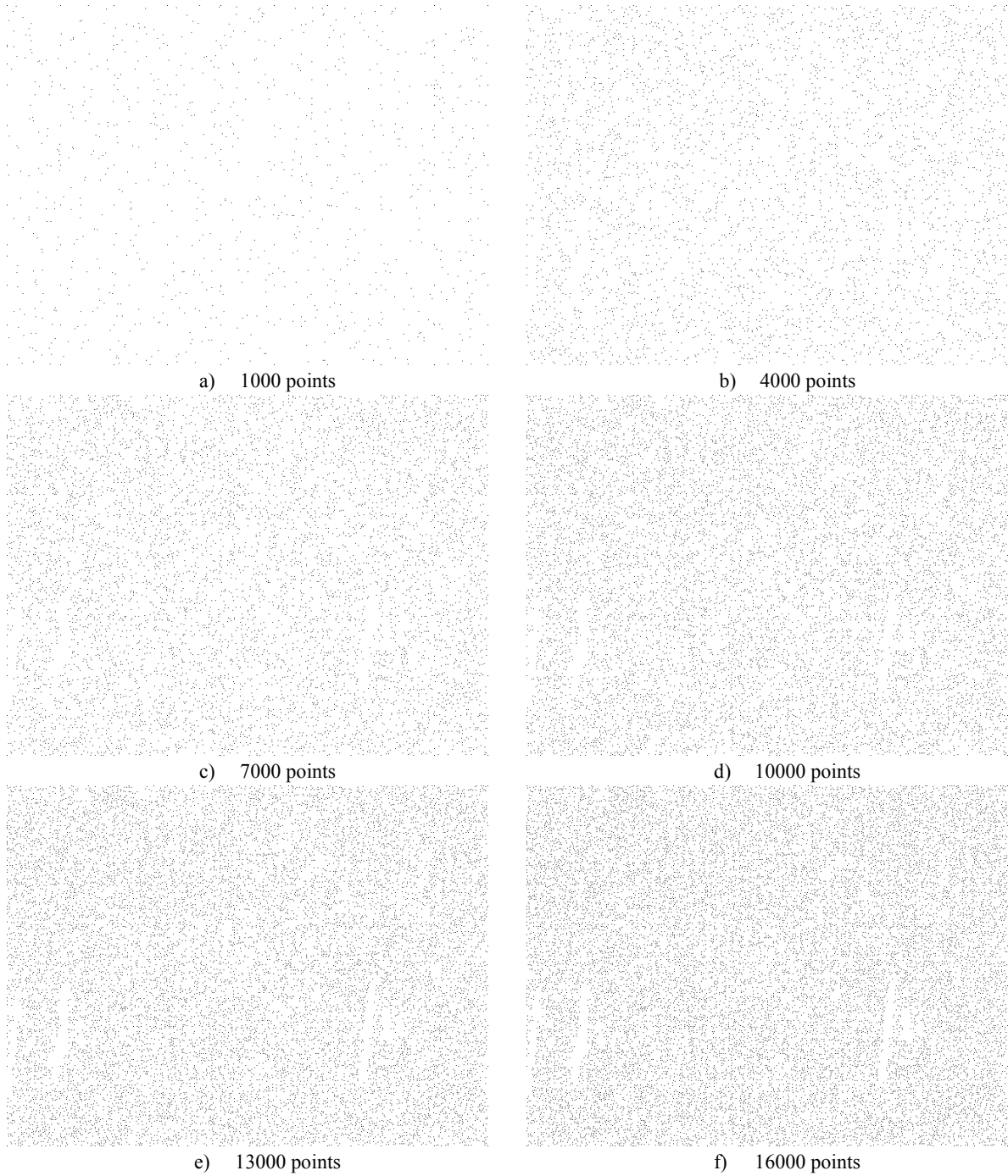
Figure 5.32 - Scene 3: point selection map progression after different numbers of points are acquired using the probabilistic occupancy grid improvement based selection process
