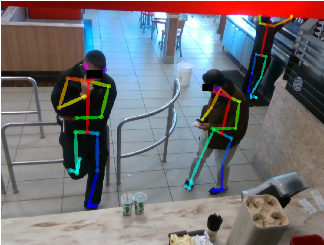
FIGURE 1.4: Human pose estimation using OpenPose
