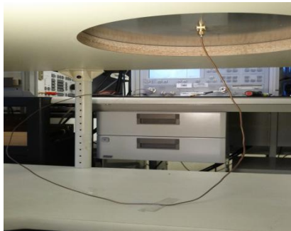
Figure 7.4 RF cable connecting VNA to the SMA connector.
