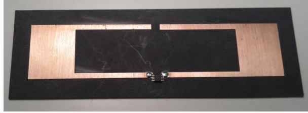
Figure 7.1c Antenna design C (Two-Wire folded dipole)
