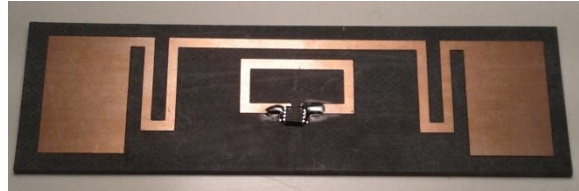
Figure 7.1d Antenna design D (Baggage tag dipole)
