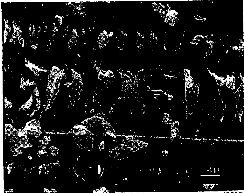
Figure 8.14 Failure surface of tubular shear specimen (2500X).
