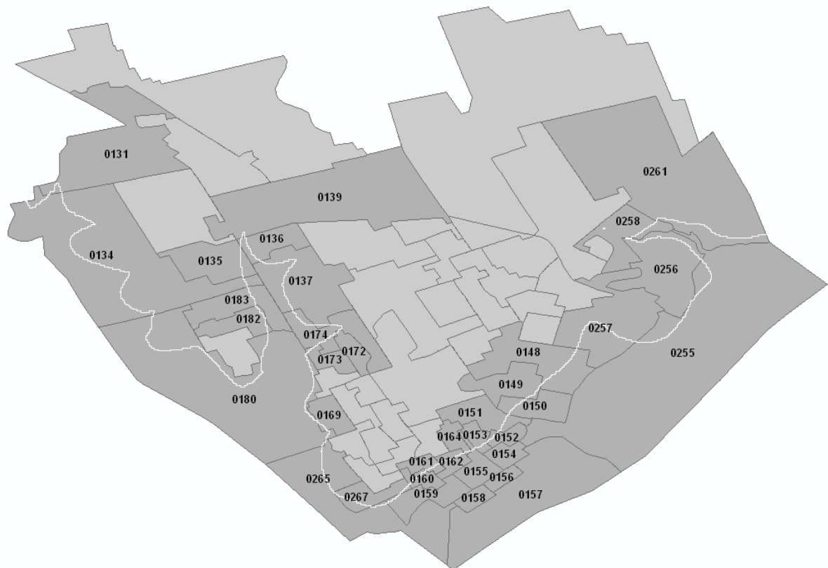
Figure 4.23: Storm Scenario VI Baseline 5 meter maximum water level flood lines on DAs (darker DAs affected by flood) (Source: Statistics Canada 2002)
