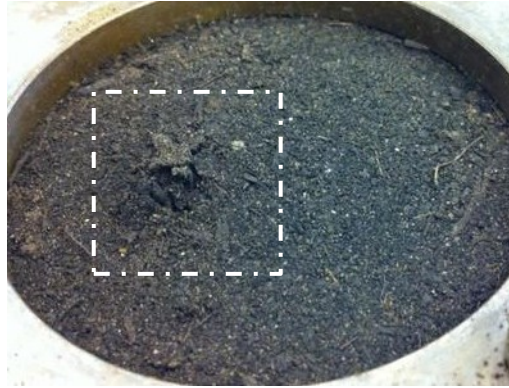
Figure 3-10 Surface change along with organic fibers at the surface of the material
