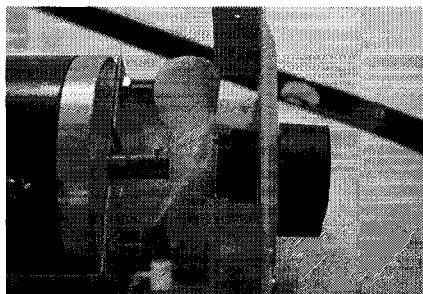
Figure 5.15: Incremental encoder mounted to pump using simple flexible coupling.
