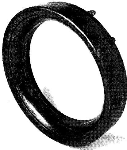
Figure 5.8: Front view of impregnation ring. The fibres are impregnated as they pass over the inner radius.
