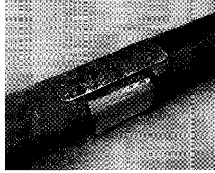
Figure 6.12: Detail of purging port in oven tube. The inner shroud prevents direct cooling of product.
