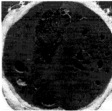
Figure 5.12: Rod cross section with voids.
