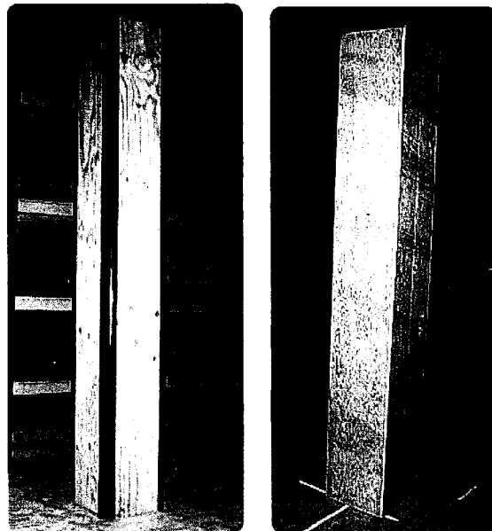
Fig. 4.3 – Templates used to manufacture FRP casings
