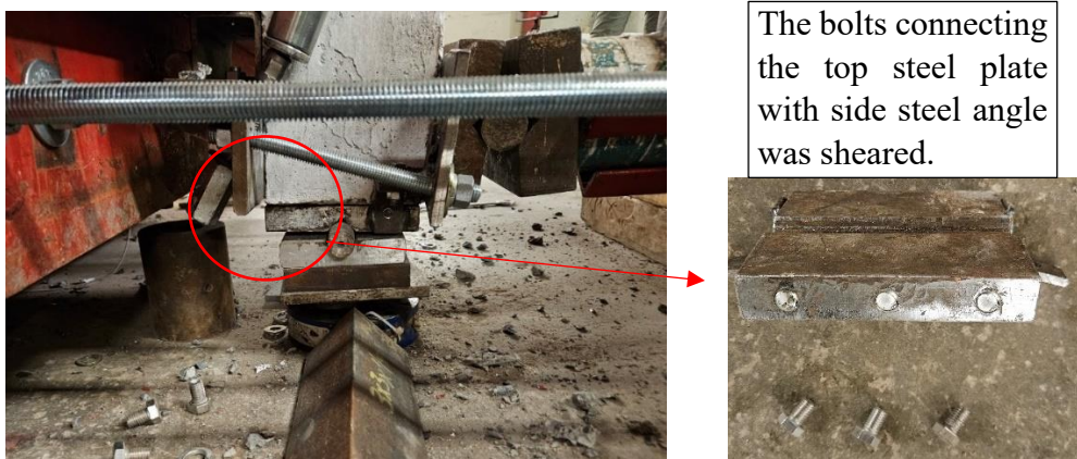
Figure 4.42 – A close-up photo of connection failure during the third shot of column P2-227e-0.16fpu-N2.
