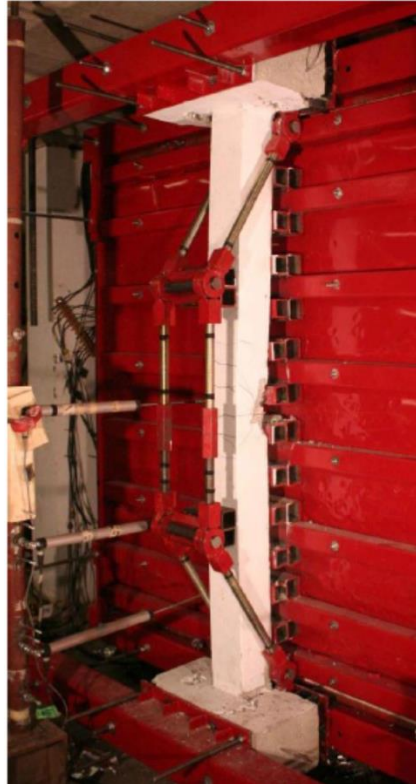
Figure 2.26 – Test result of two retrofitting methods after 4th blast shot: a) hoop prestressed column, b) tension braced column (source: [9]).
