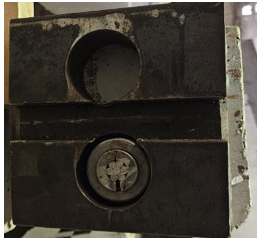
Figure 3.25 – Photos of post-tensioning of columns with internal prestressing strands: a) column with double strands during jacking, b) end of the columns with one and two strands and a thick hollow cap to facilitate axial load application during testing.
