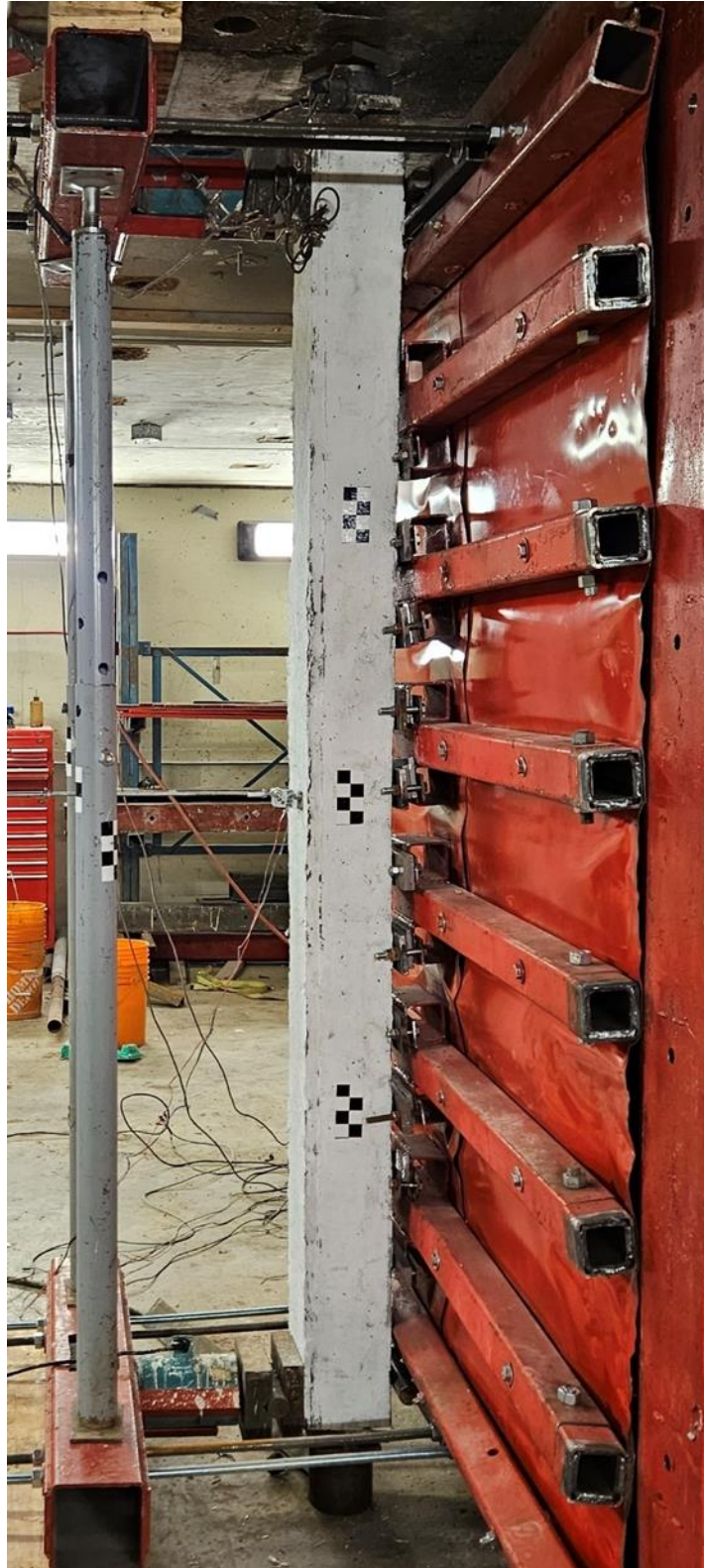
Figure 3.28 – Photo of a column prior to testing, representative of internally post-tensioned and jacketed columns.
