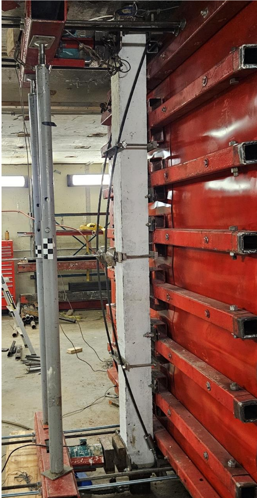
Figure 3.17 – Photo of a column with triple-harped profile prior to testing.
