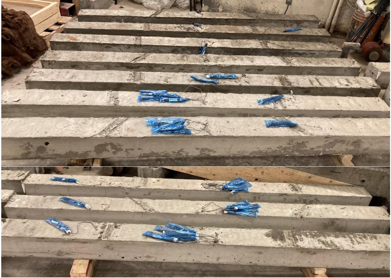
Figure 3.4 – Columns after curing; ready for strengthening/hardening and testing.
