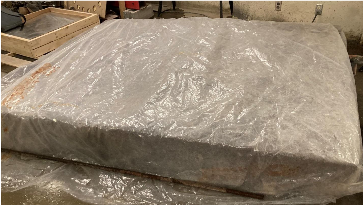
Figure 3.3 – Curing of columns with wet burlaps and polyethylene sheets.
