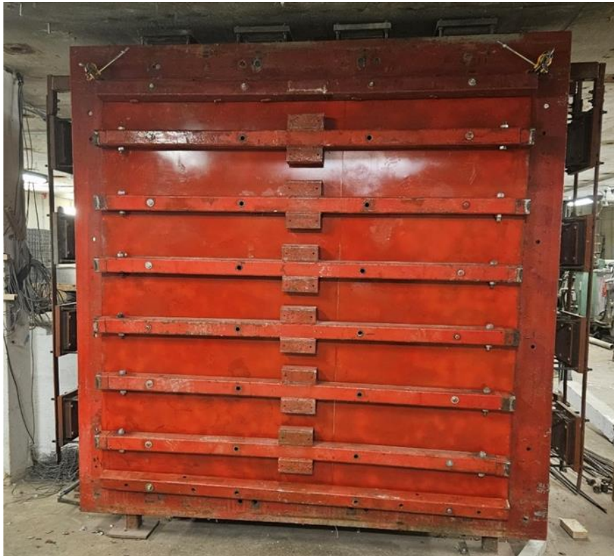
Figure 3.39 – Photos from the process of installing LTD and its stiffeners in the form of HSS.
