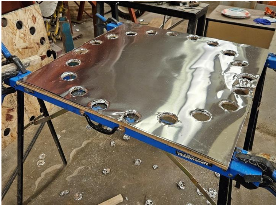
Figure 3.36 – Photos from the process of preparing diaphragms from aluminum foils.
