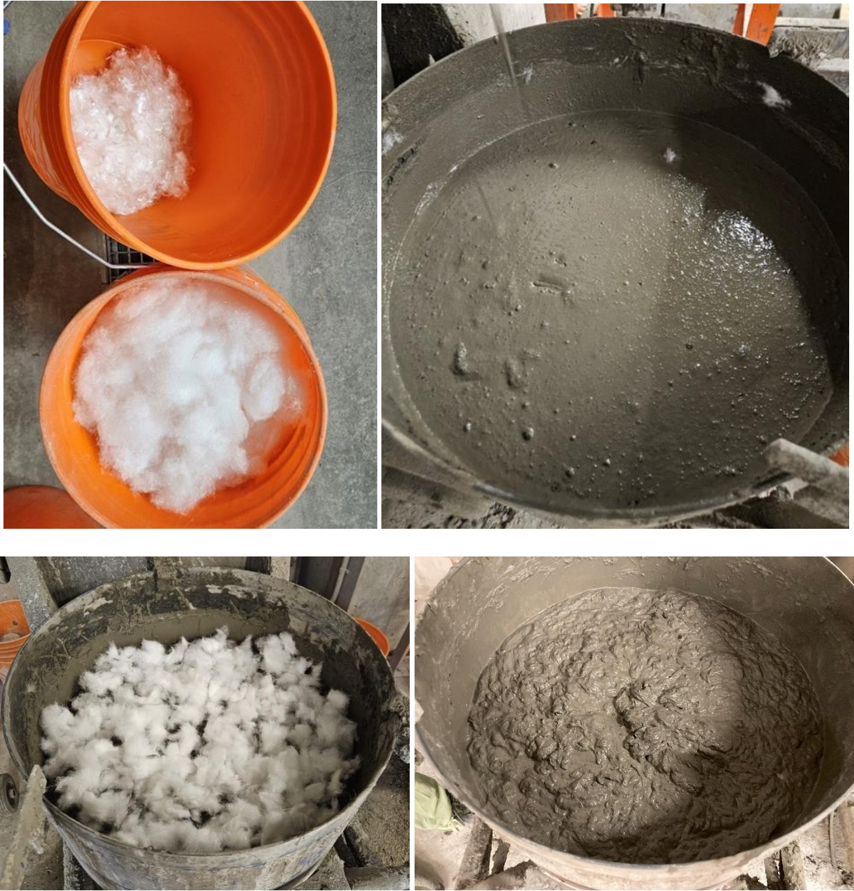
Figure 3.5 – Batching process of ECC mix.
