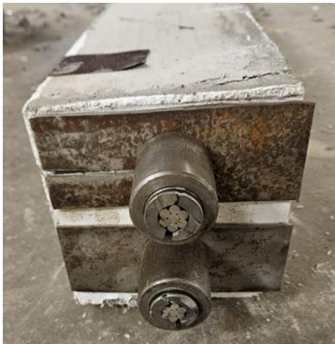
Figure 3.25 – Photos of post-tensioning of columns with internal prestressing strands: a) column with double strands during jacking, b) end of the columns with one and two strands and a thick hollow cap to facilitate axial load application during testing.
