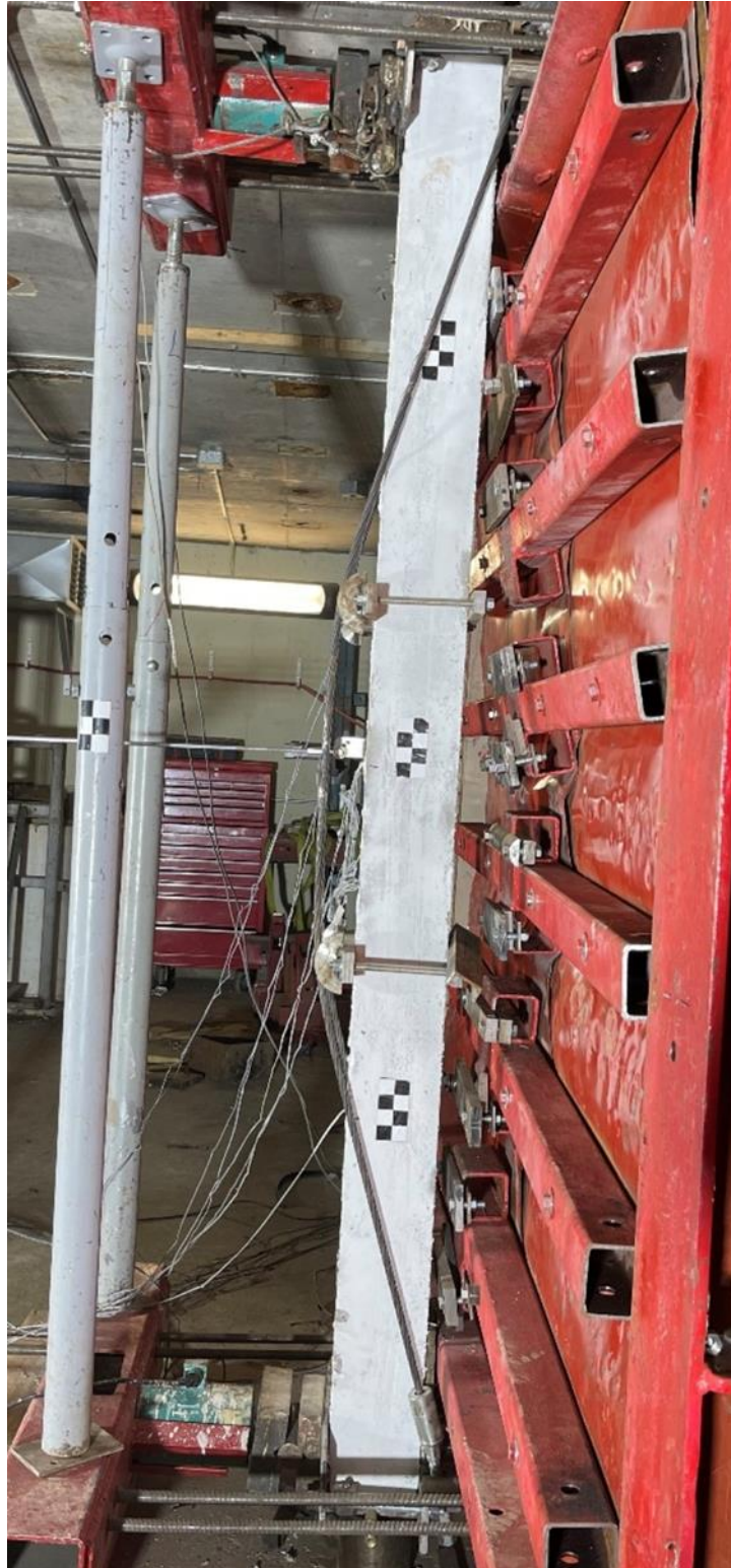
Figure 3.15 – A photo of a column with double-harped profile prior to testing.
