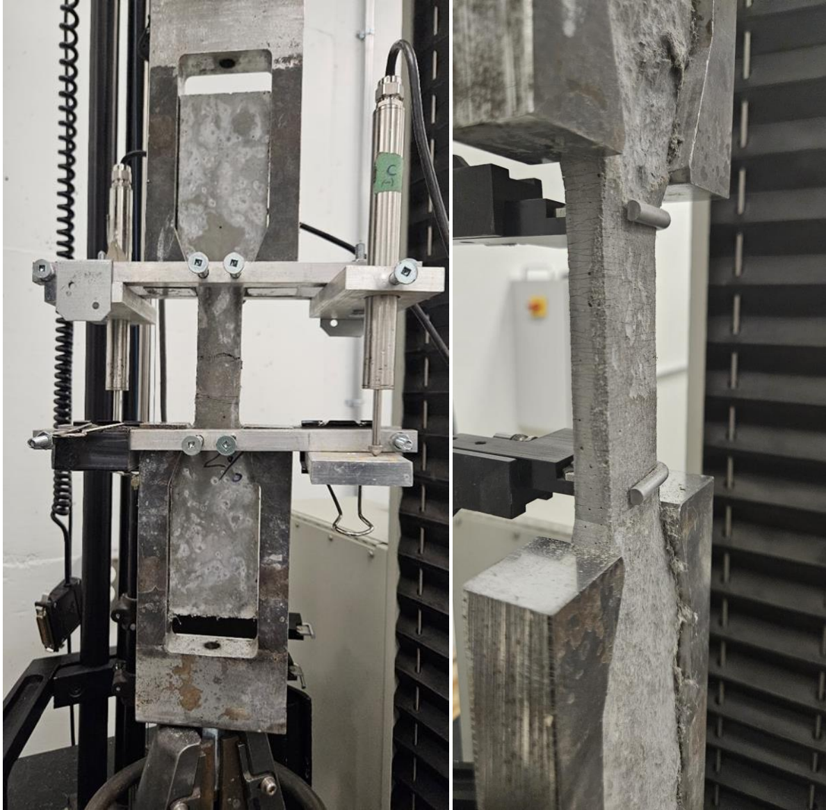
Figure 3.6 – ECC dog-bone coupon test setup and a close-up photo of a coupon with 2% polyethylene fibers.
