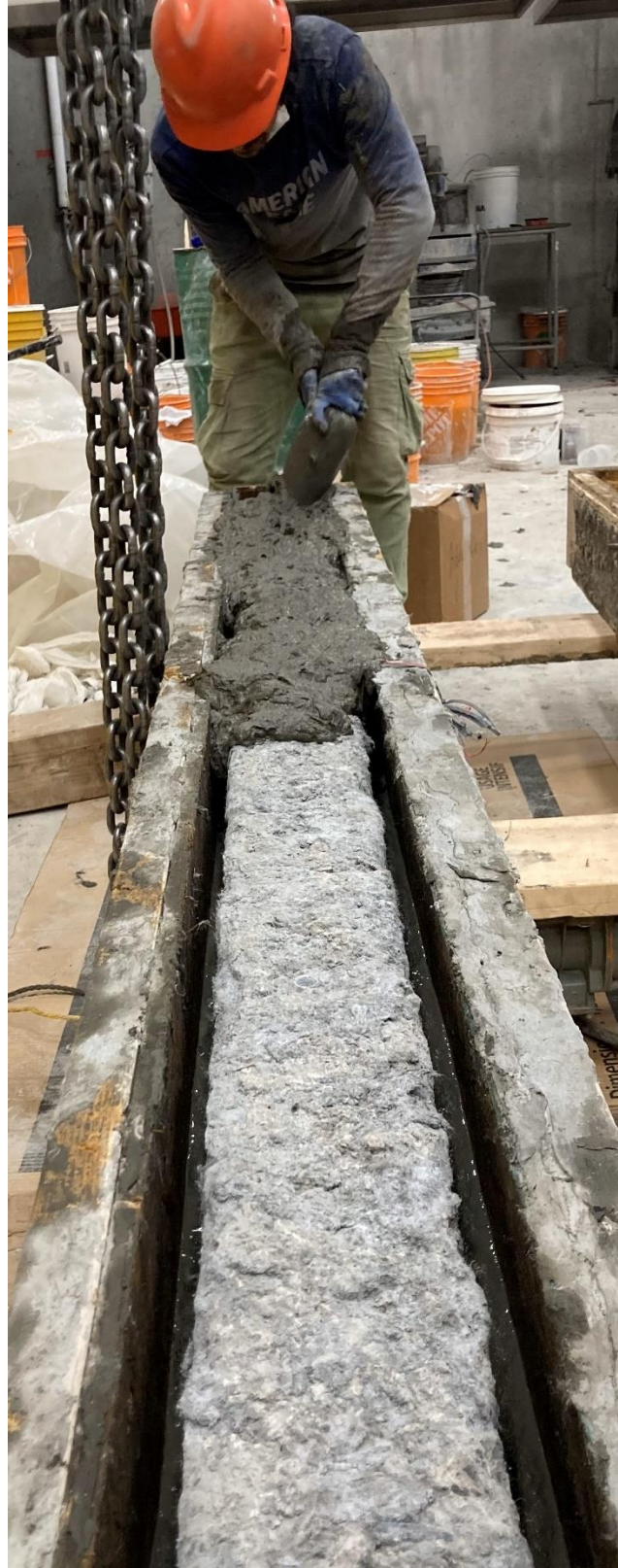
Figure 3.30 – A photo taken while pouring the ECC layer on all surfaces of the column core for ECC jacketed columns.
