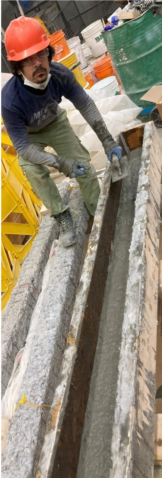
Figure 3.30 – A photo taken while pouring the ECC layer on all surfaces of the column core for ECC jacketed columns.
