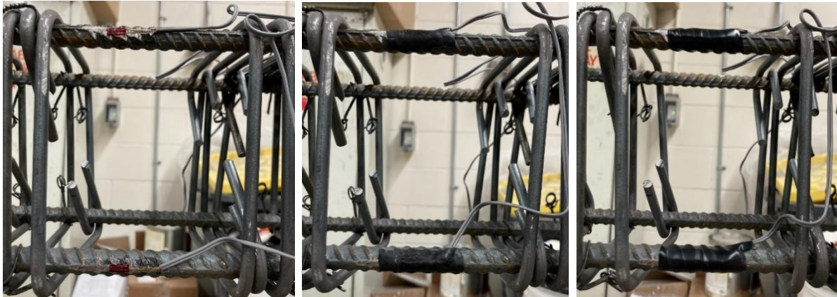
Figure 3.32 – A photo illustrating strain gauges on longitudinal and transverse reinforcement.
