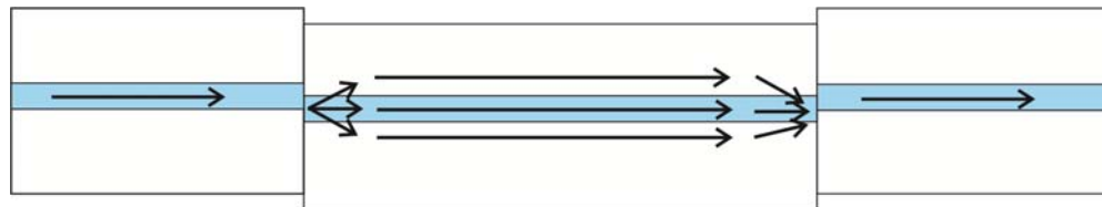
Figure 2.4 A schematic profile of core-offset fiber Mach-Zehnder interferometer
