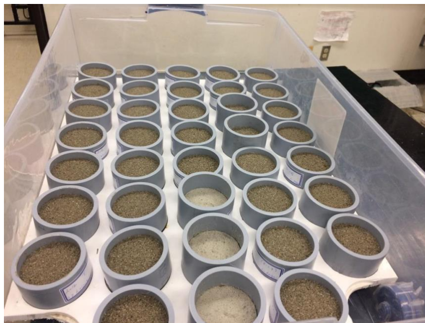
Figure 5.4. Compacted specimens placed in a water reservoir for inundation
