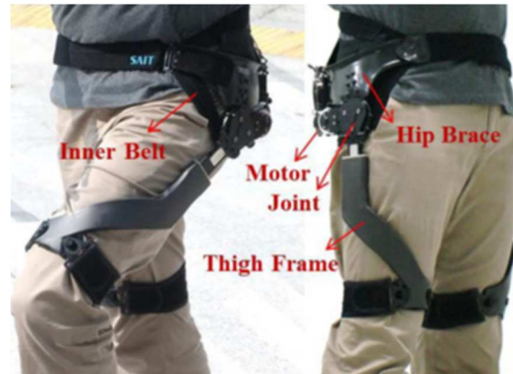
Figure 2.2. The Gait Enhancing Mechatronic System (GEMS) hip assist robot [17]. Copyright © 2017, IEEE; used with permission.
