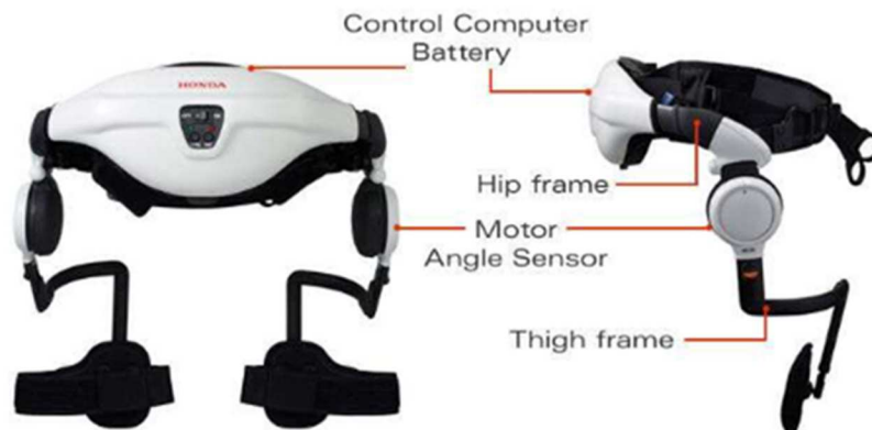
Figure 2.6. Honda's walking assist device [20]. Copyright© 2015, Buesing et al.; used with permission.
