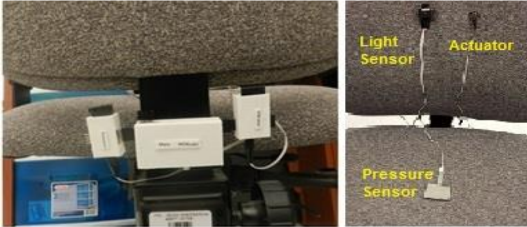
Figure 5.4 The smart office chair scenario, the hardware prototype composed of the mainboard, pressure and light sensors, and vibrotactile actuator
