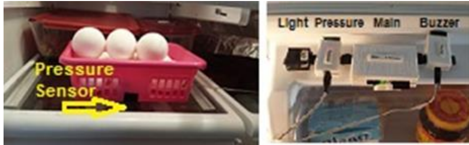
Figure 5.5 The smart fridge scenario, (Left) a pressure sensor located underneath the eggs container. (Right) the mainboard, light sensor, and buzzer are appended on the fridge door
