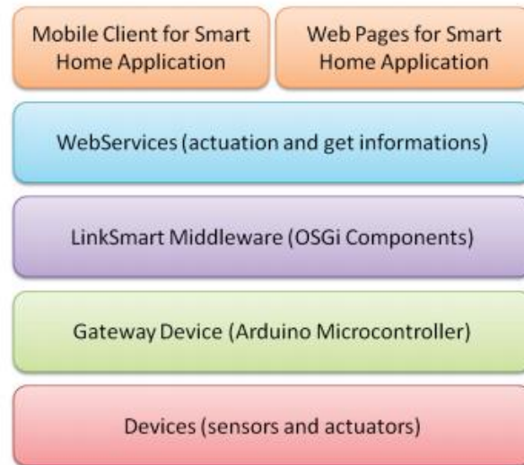
Figure 2.2 Layered architecture of the smart home application [11]
