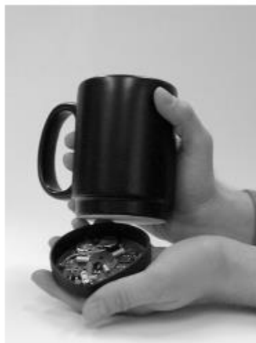
Figure 2.6 The Mediacup is an ordinary coffee cup with sensors, processing, and communication embedded in the base [40]
