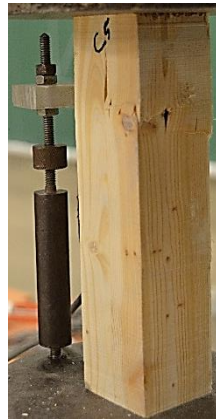
(c) Compression failure
