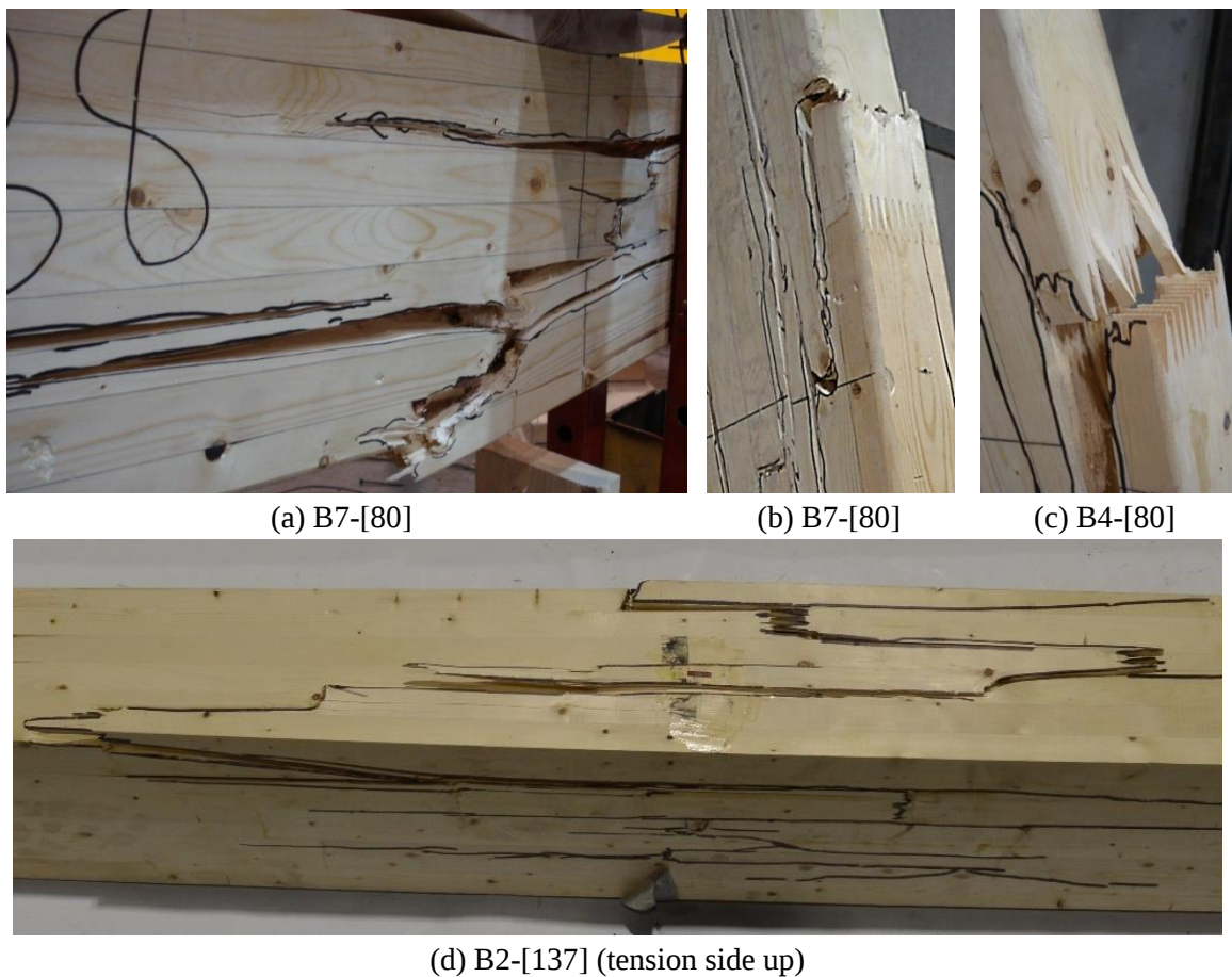
Figure 4.5: Representative static failure modes of glulam beams
