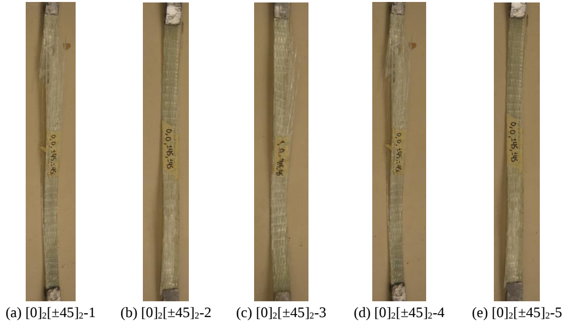
Figure B.20: Representative failure modes for GFRP [0]_2[\pm 45]_2
