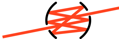
Figure 16: Herriott cell with entrance and exit holes on opposite mirrors
