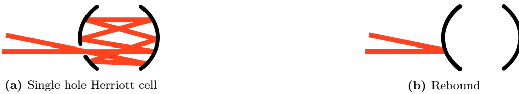
Figure 15: Intuition for the behaviour of a single entrance and exit hole Herriott cell
