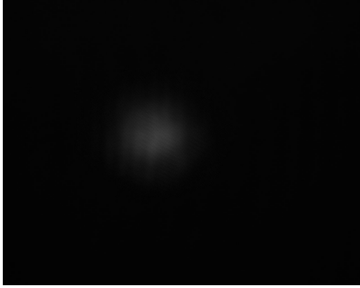
(a) HG00 mode as recorded by the camera after an HC with total delay of 7.9 m
