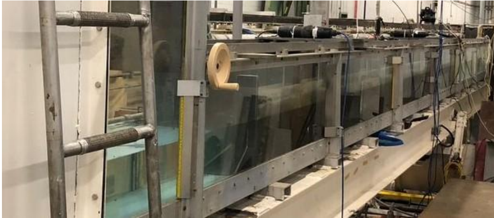
Figure 15. NRC-OCRE Tilting flume adapted from Bigdeli et al. (2024)
