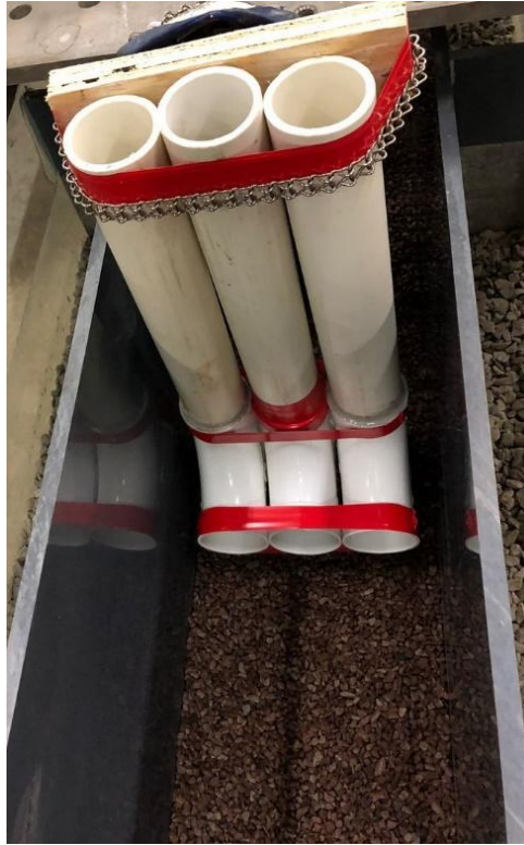
Figure 7. Injection tubes across the channel's width.
