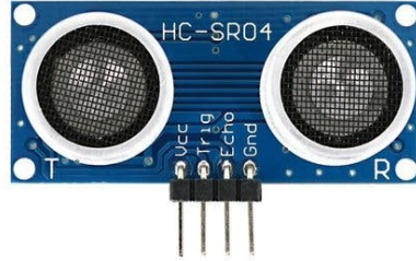
Figure 3.21: Ultrasonic sensor used on Alphabot2
