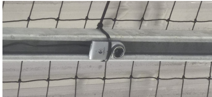
(b) Webcam attached to metal beam above the robotic agents
