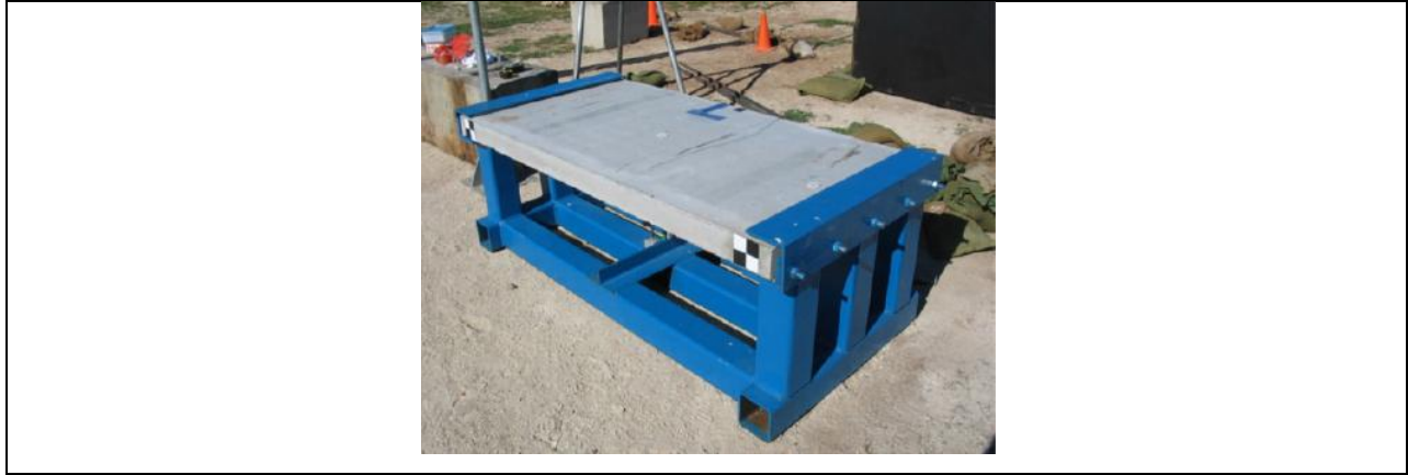
Figure 2.5 Slab with test fixture
