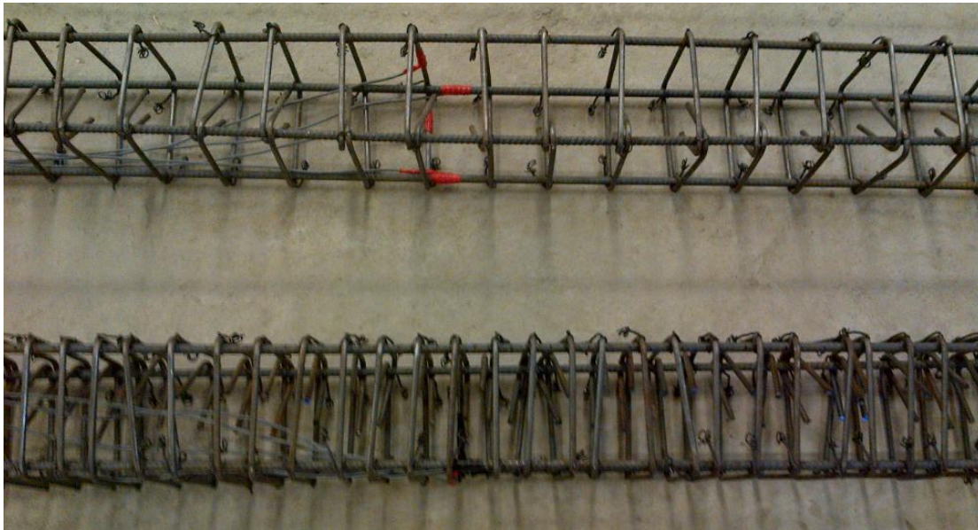
Figure 3.6 Non-seismic (top) vs. Seismic (bottom) detailing
