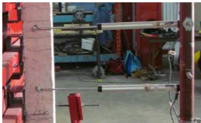
Figure 3.16 LVDT connection to column (left) and support post (right)
