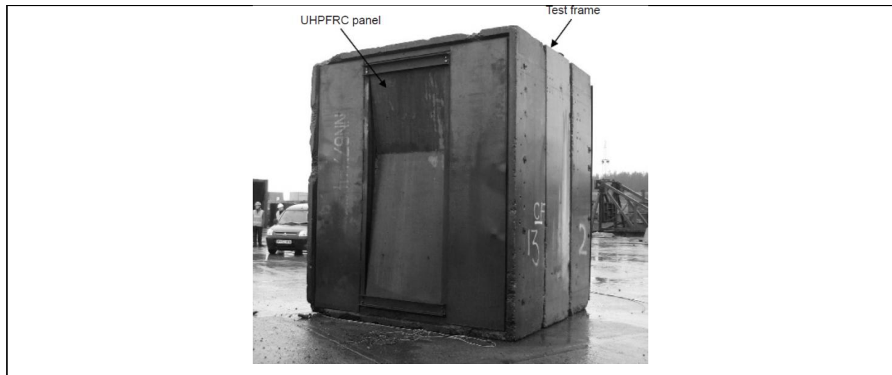
Figure 2.6 Panel after testing
