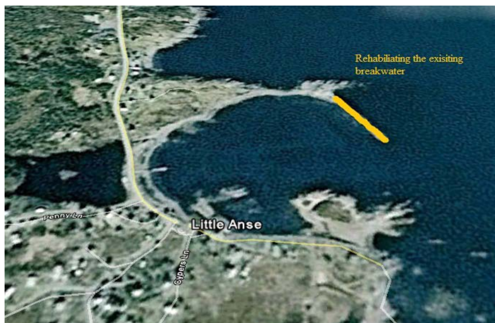
Figure 5.7: Rehabilitating the existing breakwater
