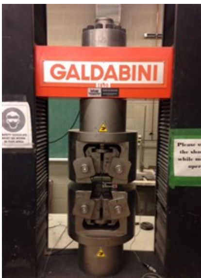
(a) GALDABINI Testing Frame
