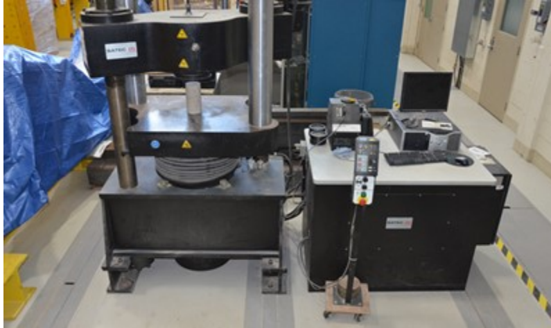
(a) SATEC 2000 KN universal testing machine with cylinder ready for testing
