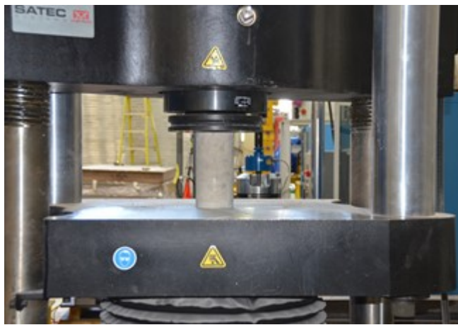
(b) Cylinder in testing compartment
