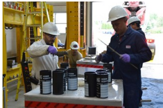
(b) Preparation of standard cylinders
