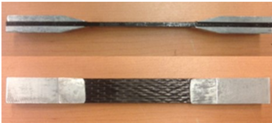
(b) Typical CFRP coupon with tabs attached
