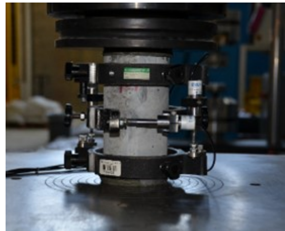
(c) Compressometer setup
