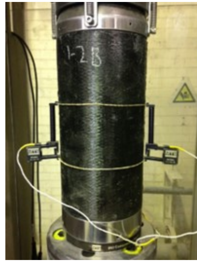
(b) 150 mm specimen with extensometers
