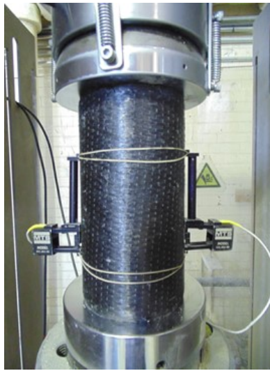
(a) 100 mm specimen with extensometers
