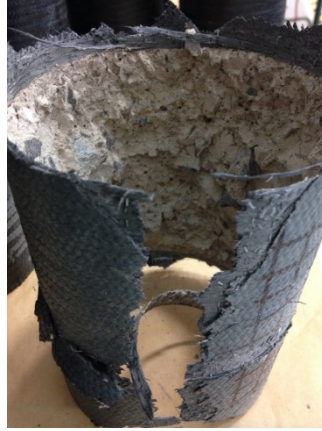
Figure 4-4 Perfect bond between concrete and CFRP jacket
