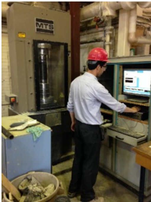
(a) MTS testing machine
