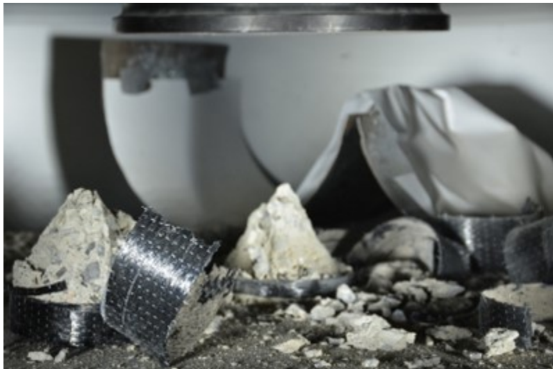
Figure 3-14 Typical explosive failure of CFRP Confined Specimens
