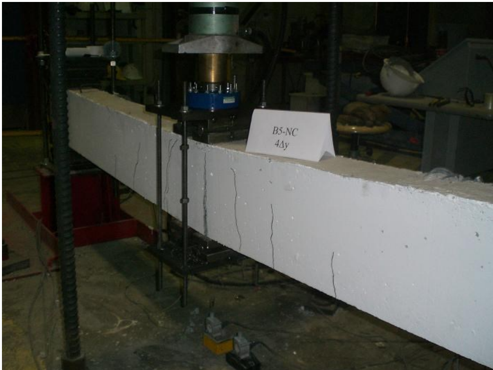
Figure F.23 B5-NC Beam After ( 4\Delta y ) Displacement
