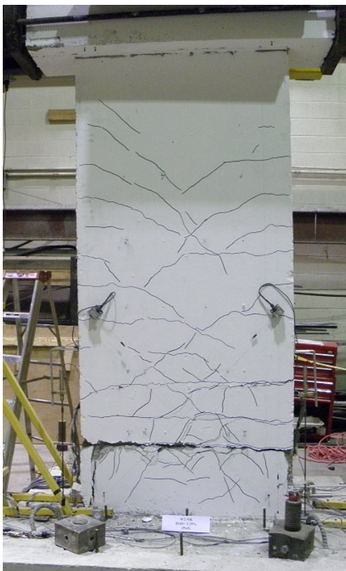
Figure 7.24 Cracking Pattern at Failure in W2-NR
