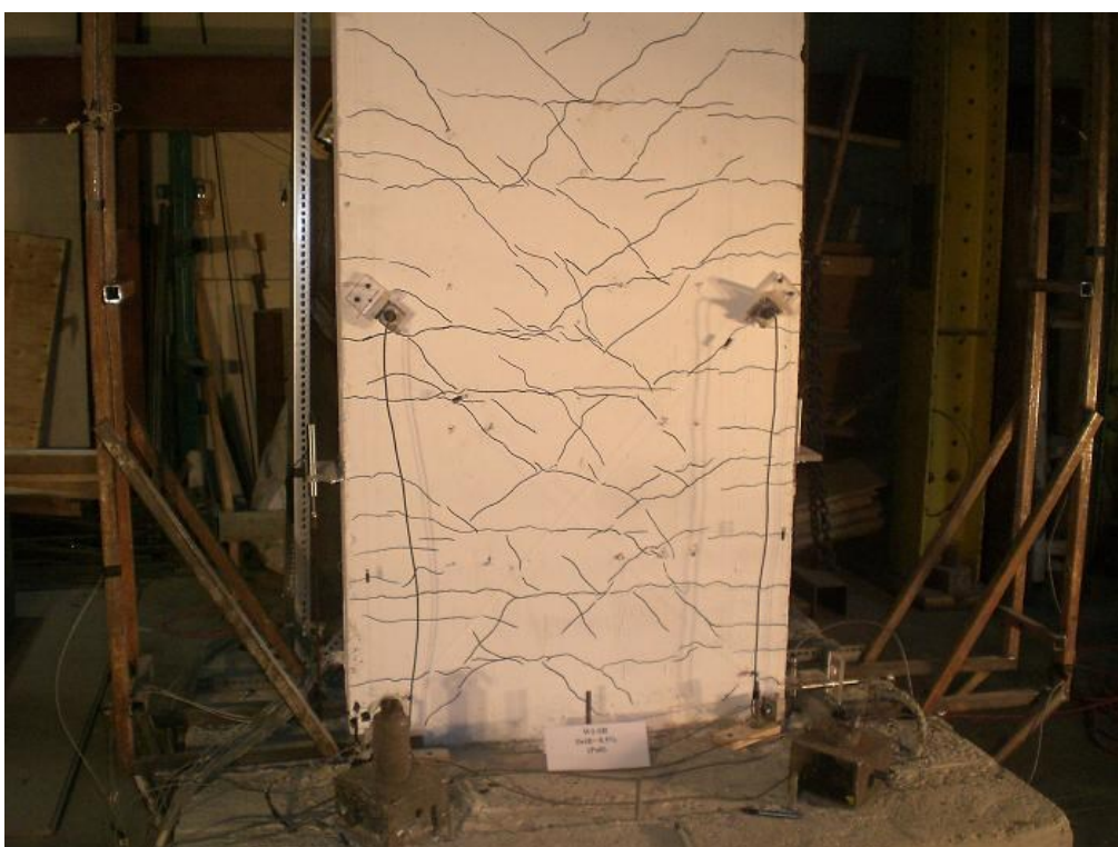
Figure F.39 W1-SR Wall After (0.75%) Drift
