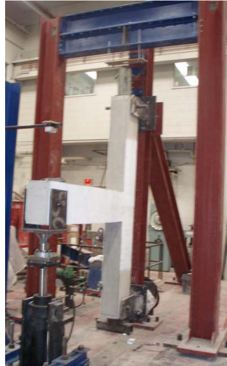
Figure 8.6 Details of Beam-Column Joint Specimen (Alam et al. 2007)
