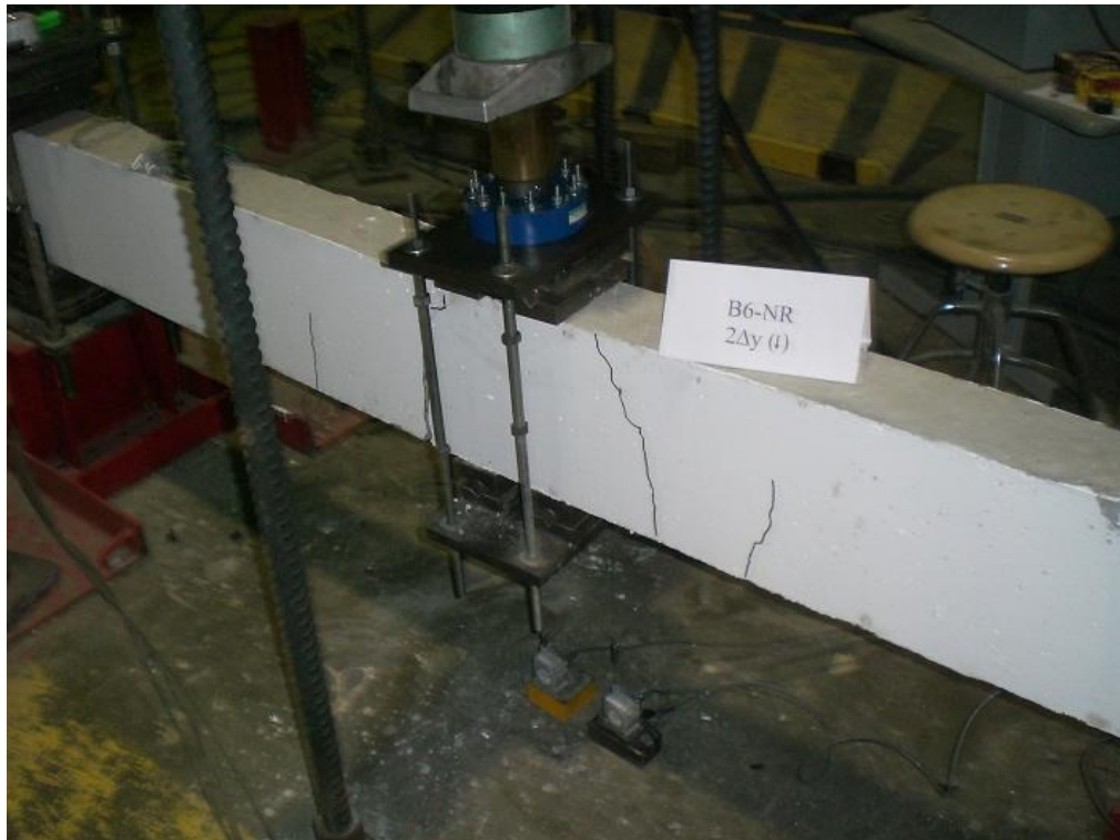
Figure F.29 B6-NR Beam After ( 2\Delta y ) Displacement
