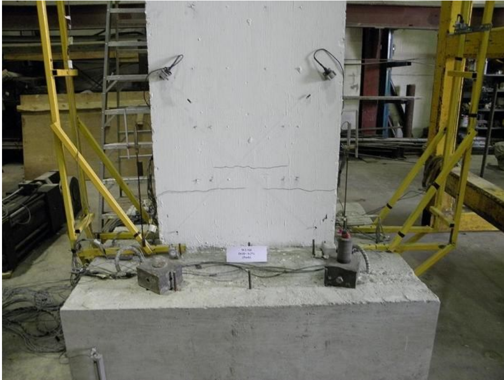
Figure F.44 W2-NR Wall After (0.2%) Drift
