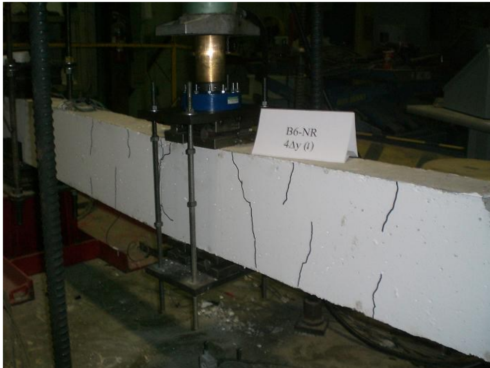
Figure F.31 B6-NR Beam After ( 4\Delta y ) Displacement
