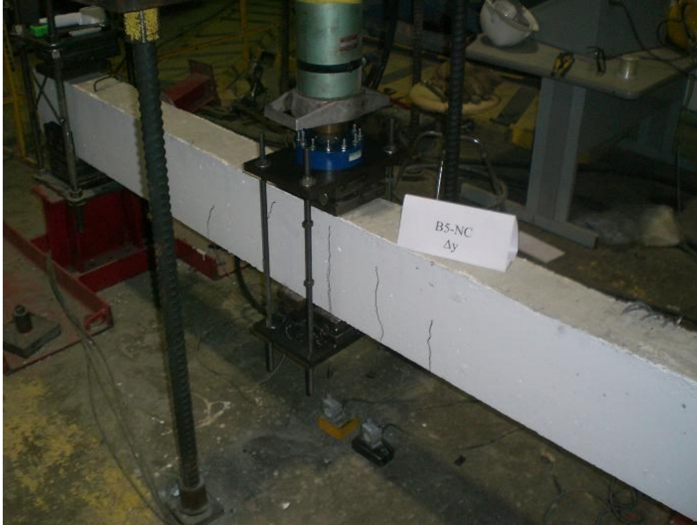
Figure F.20 B5-NC Beam After ( \Delta y ) Displacement
