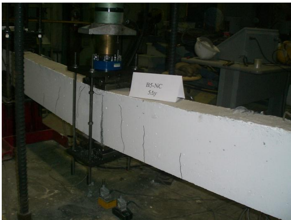
Figure F.24 B5-NC Beam After ( 5\Delta y ) Displacement
