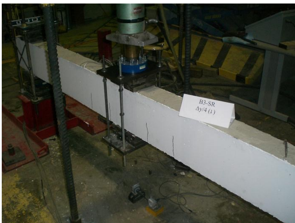
Figure F.9 B3-SR Beam After ( \Delta y/4 ) Displacement
