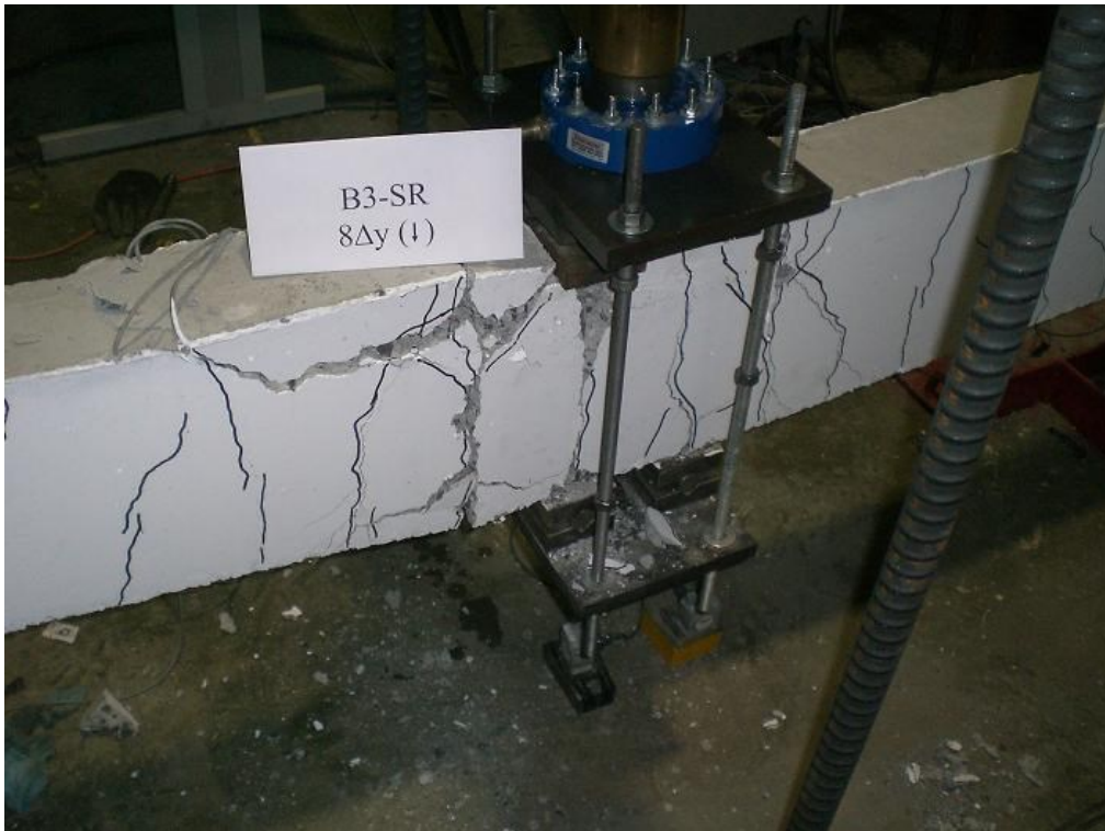
Figure F.17 B3-SR Beam After ( 8\Delta y ) Displacement
