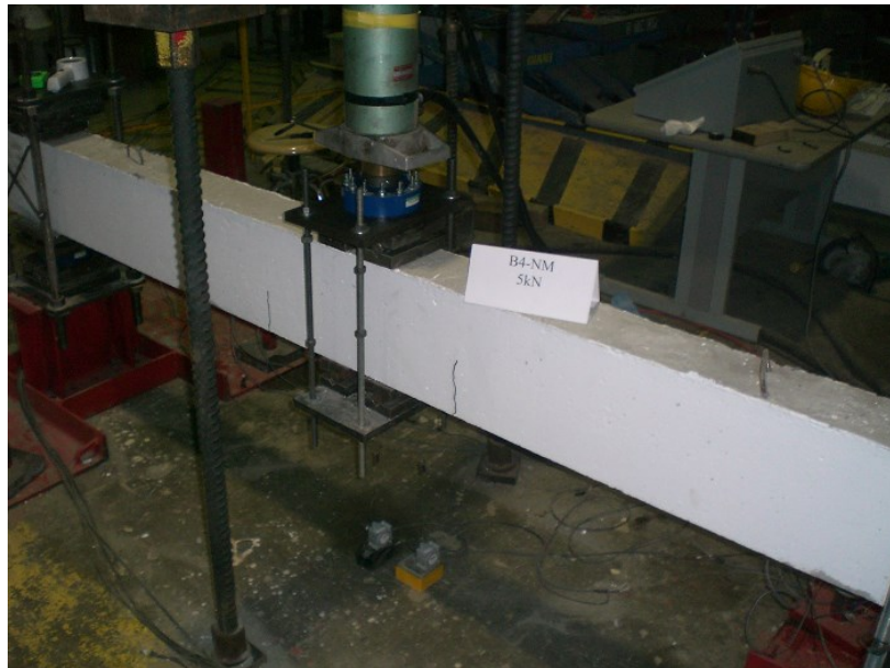
Figure 3.20 Loading and Displacement Setup
