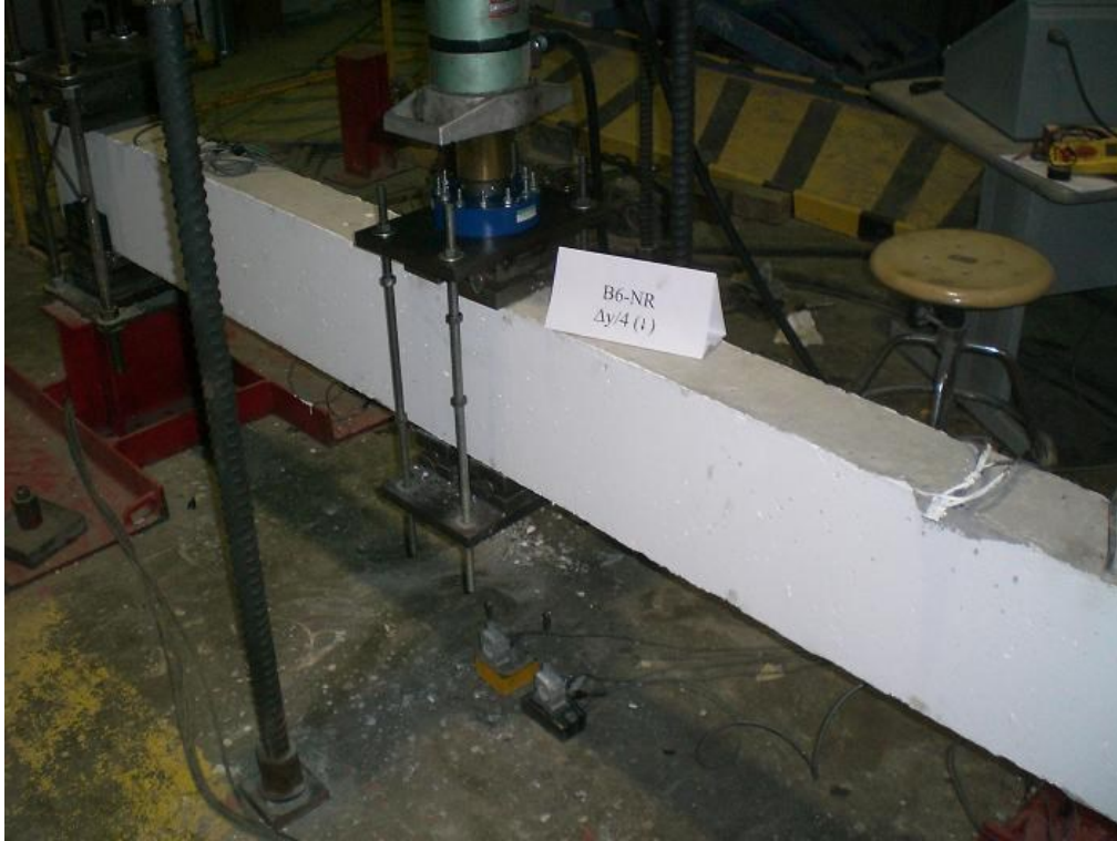
Figure F.26 B6-NR Beam After ( \Delta y/4 ) Displacement
