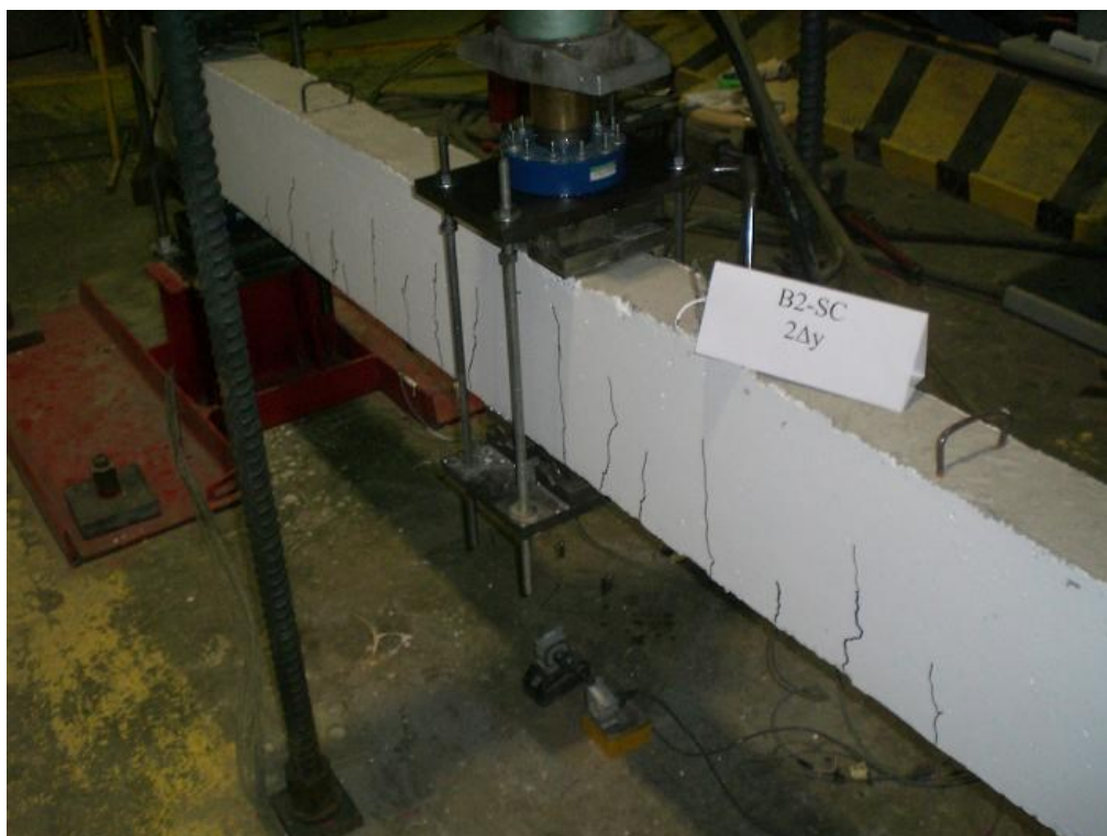
Figure F.4 B2-SC Beam After ( 2\Delta y ) Displacement
