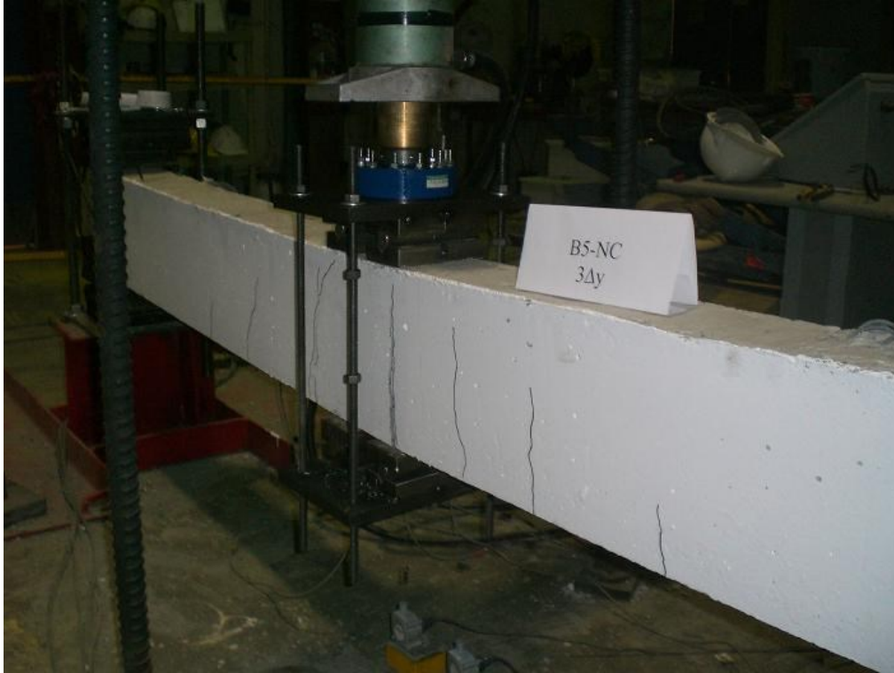
Figure F.22 B5-NC Beam After ( 3\Delta y ) Displacement
