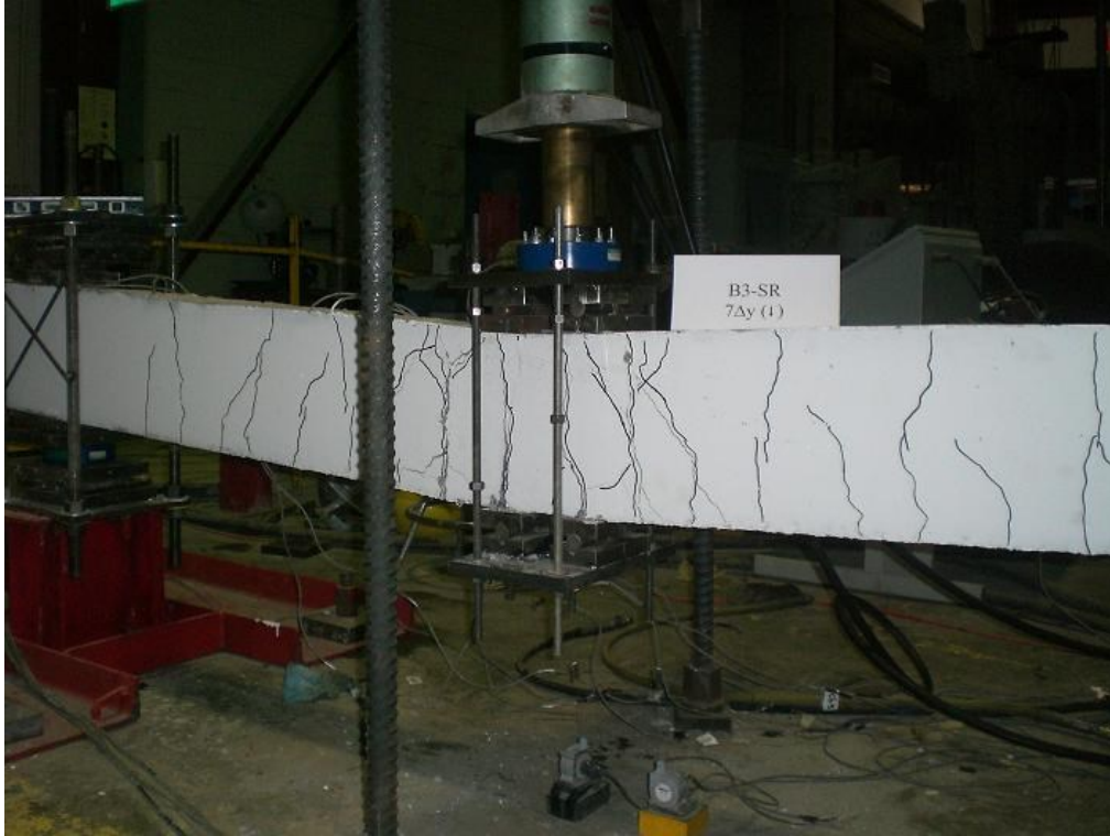
Figure F.16 B3-SR Beam After ( 7\Delta y ) Displacement
