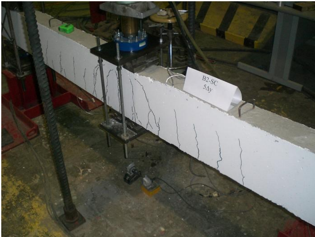
Figure F.7 B2-SC Beam After ( 5\Delta y ) Displacement
