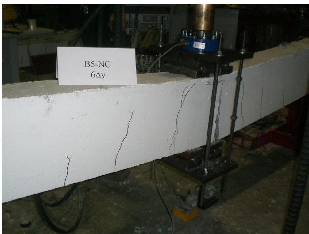
Figure F.25 B5-NC Beam After ( 6\Delta y ) Displacement
