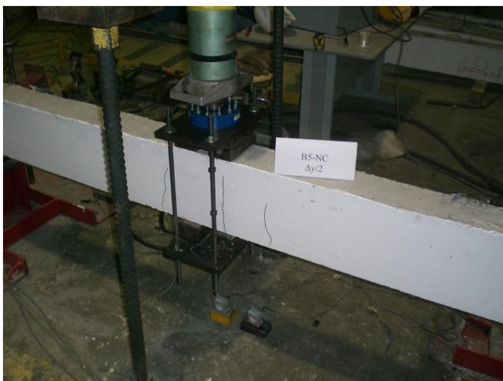
Figure F.19 B5-NC Beam After ( \Delta y/2 ) Displacement
