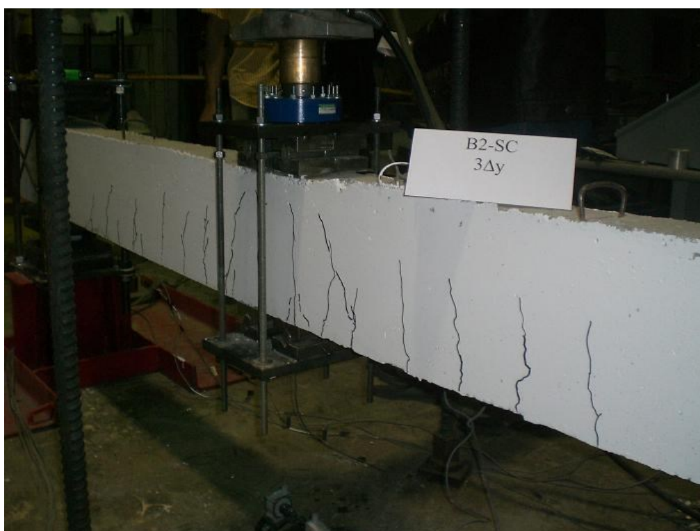
Figure F.5 B2-SC Beam After ( 3\Delta y ) Displacement
