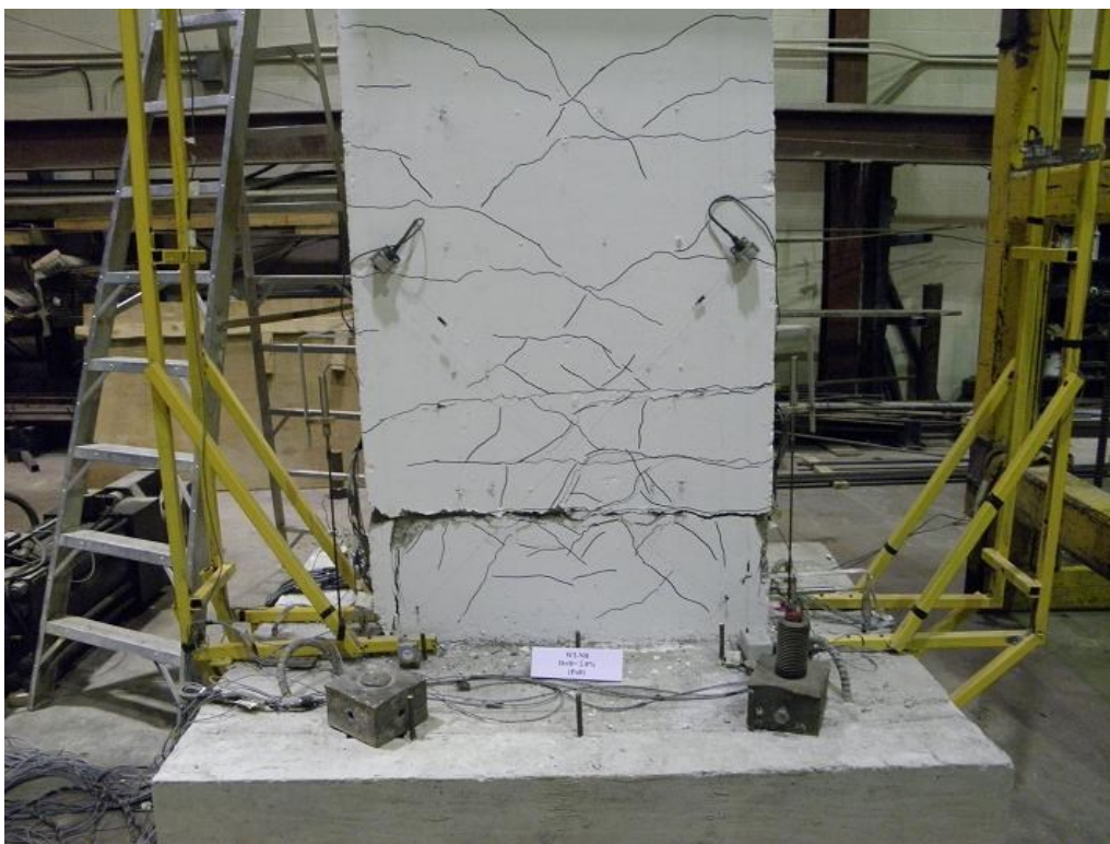
Figure F.52 W2-NR Wall After (2%) Drift
