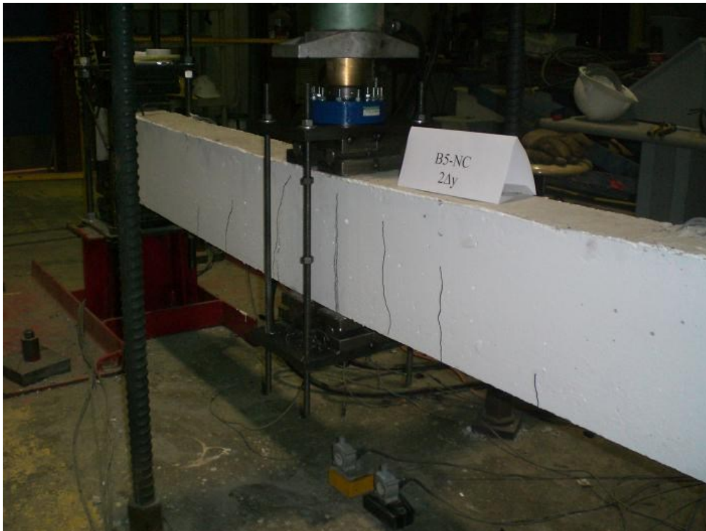
Figure F.21 B5-NC Beam After ( 2\Delta y ) Displacement
