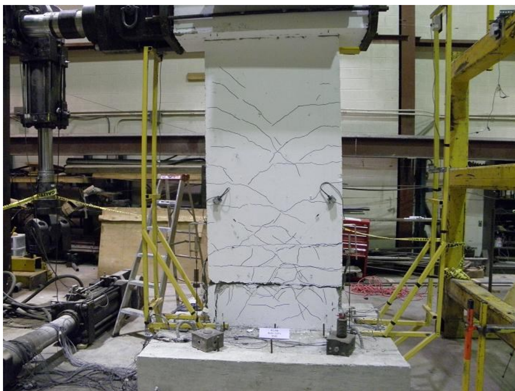
Figure F.53 W2-NR Wall After (2.25%) Drift
