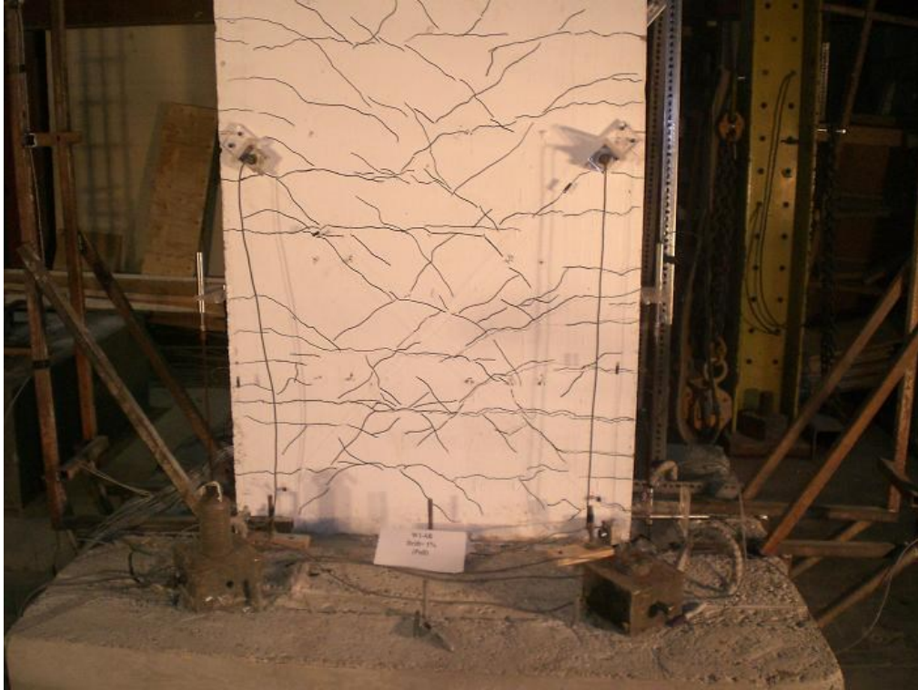
Figure F.40 W1-SR Wall After (1%) Drift
