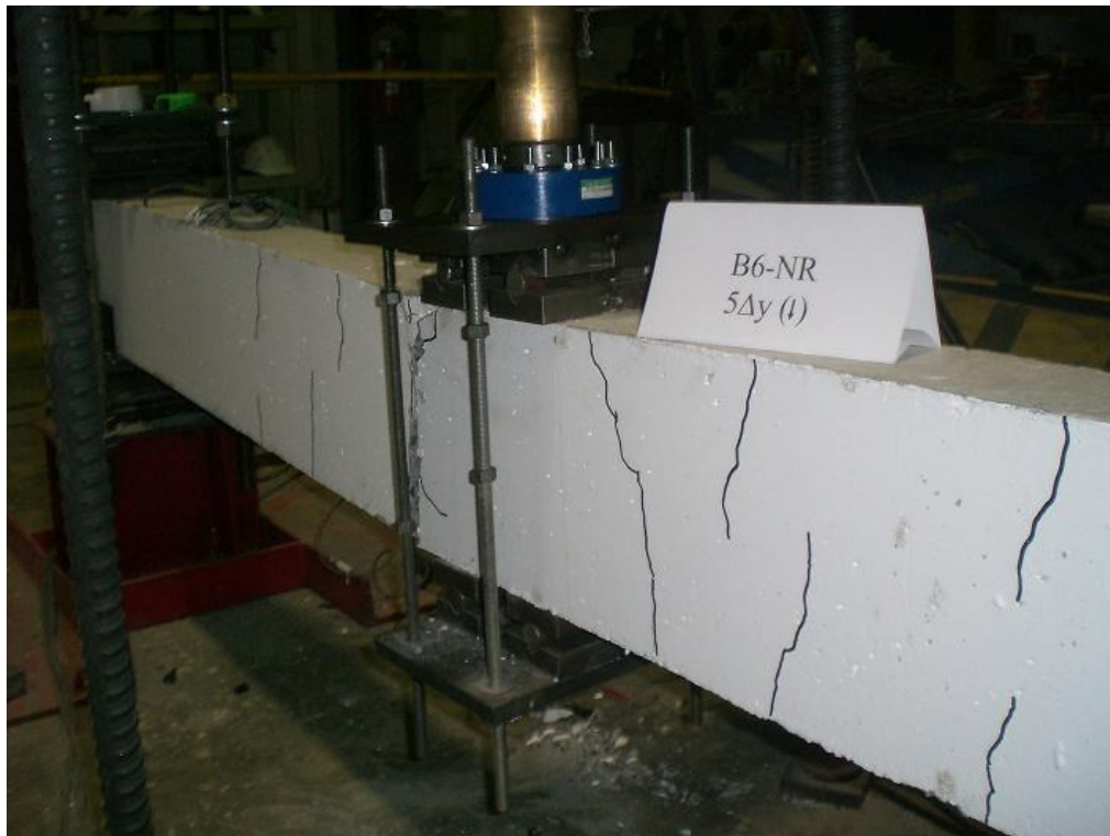
Figure F.32 B6-NR Beam After ( 5\Delta y ) Displacement
