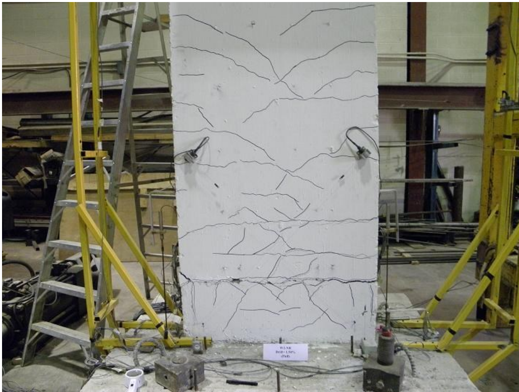
Figure F.50 W2-NR Wall After (1.5%) Drift
