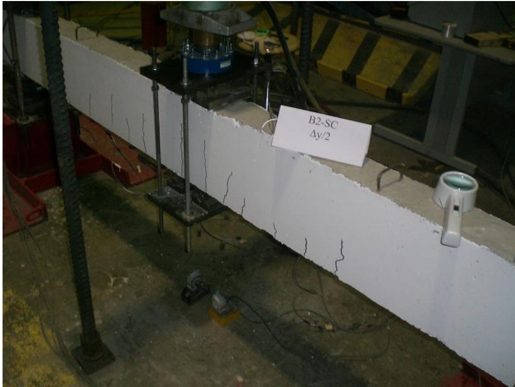
Figure F.2 B2-SC Beam After ( \Delta y/2 ) Displacement
