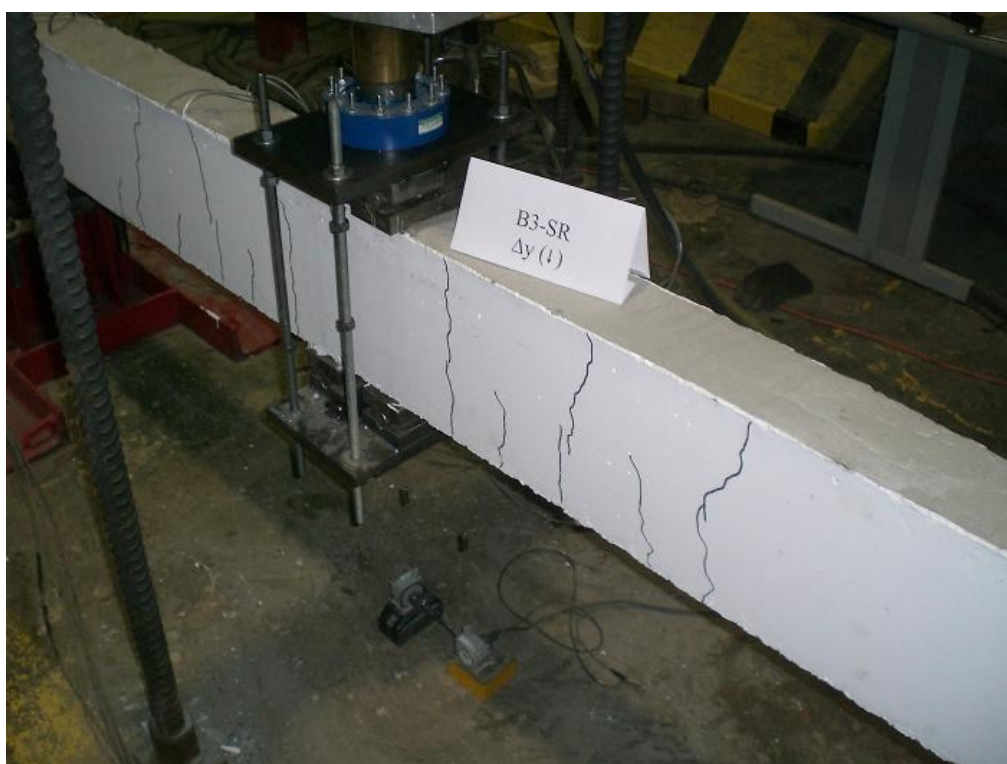
Figure F.11 B3-SR Beam After ( \Delta y ) Displacement
