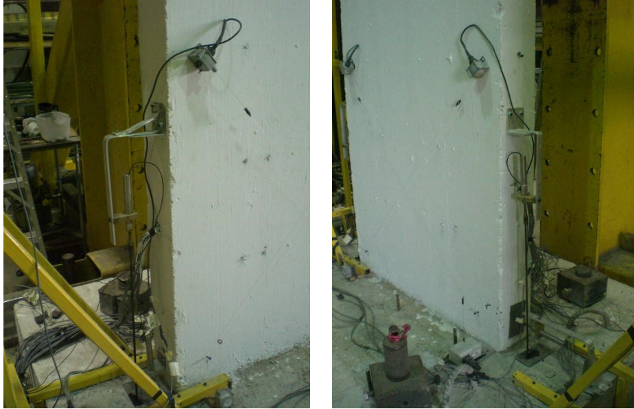
Figure 3.28 Location of LVDTs Near Wall Base
