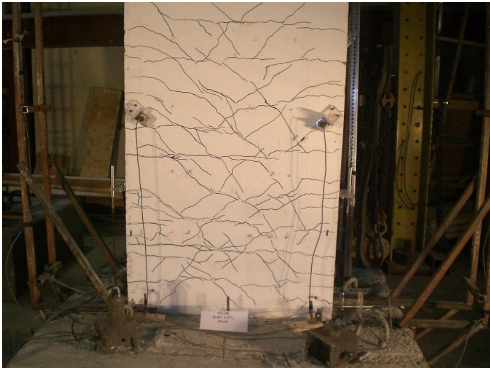
Figure F.41 W1-SR Wall After (1.25%) Drift
