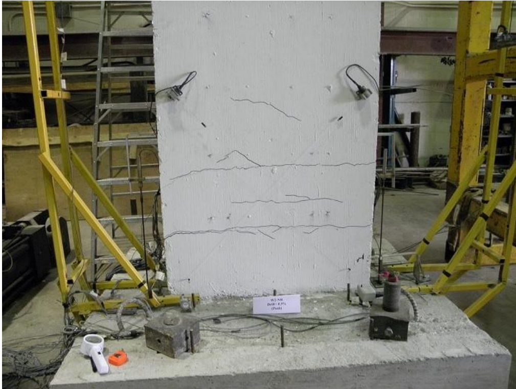
Figure F.46 W2-NR Wall After (0.5%) Drift
