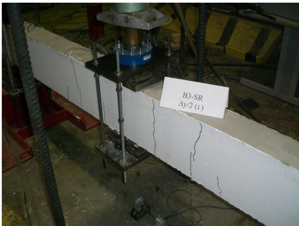
Figure F.10 B3-SR Beam After ( \Delta y/2 ) Displacement
