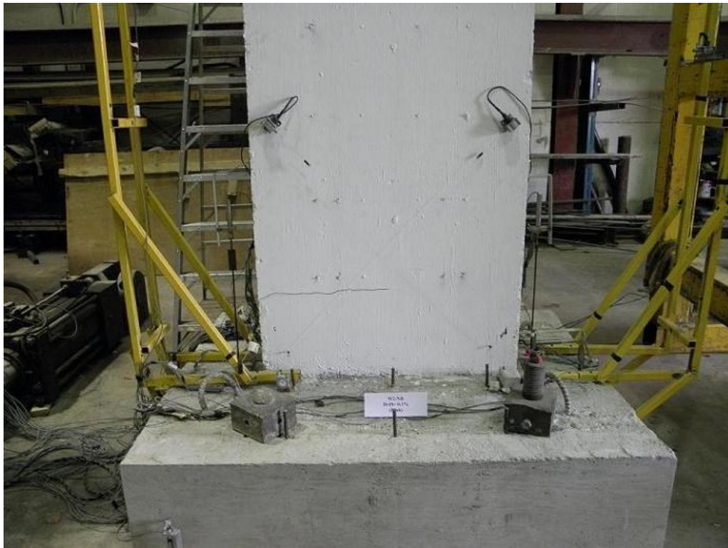
Figure F.43 W2-NR Wall After (0.1%) Drift
