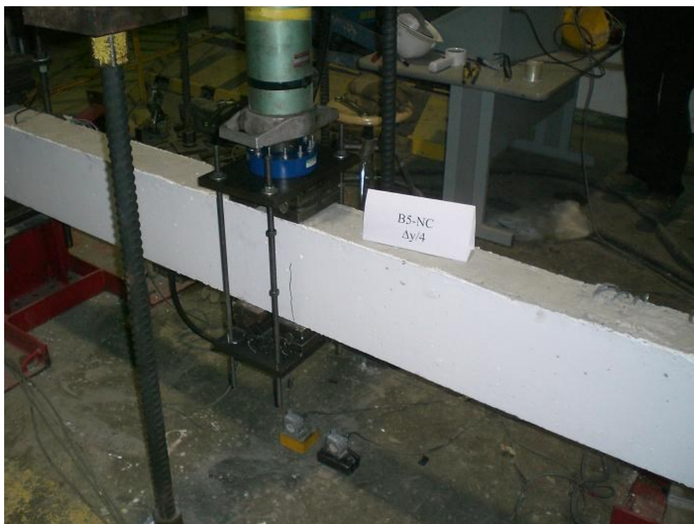
Figure F.18 B5-NC Beam After ( \Delta y/4 ) Displacement
