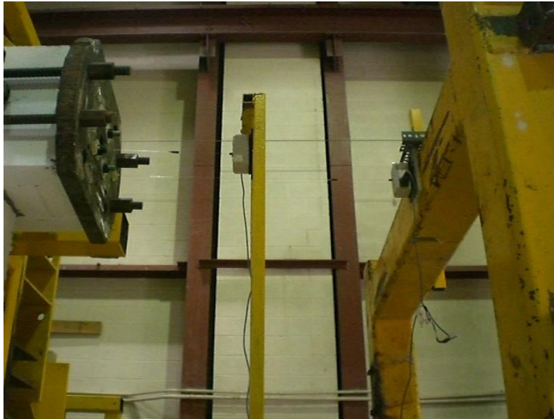
Figure 3.27 Location of DCTs for Top Beam Lateral Displacement
