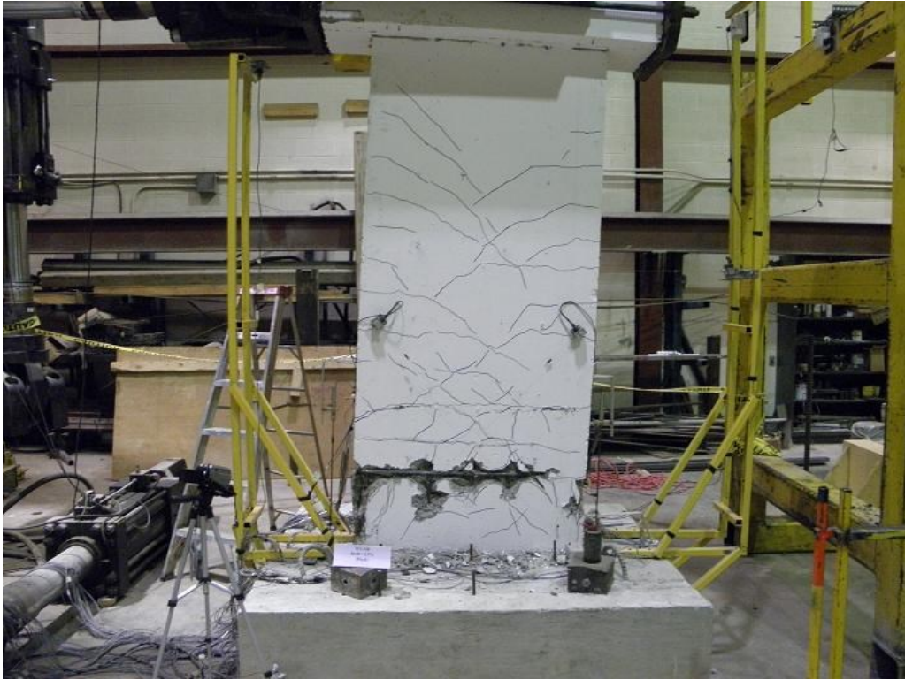
Figure F.56 W2-NR Wall After (3.5%) Drift
