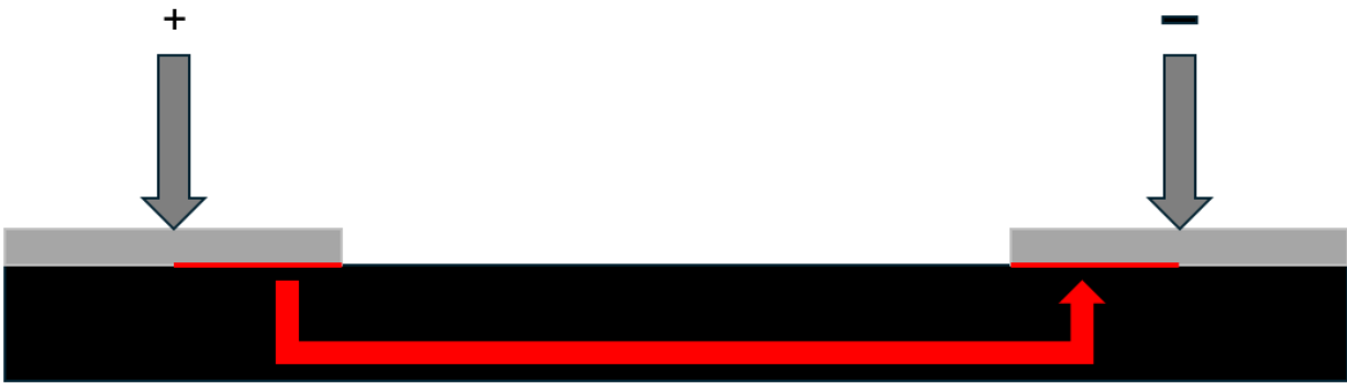
Figure 2.20: Current crowding effect for planar structures. Despite the fact that the metal contact pad is much larger, most of the current flows through the edge of the contact (highlighted in red).
