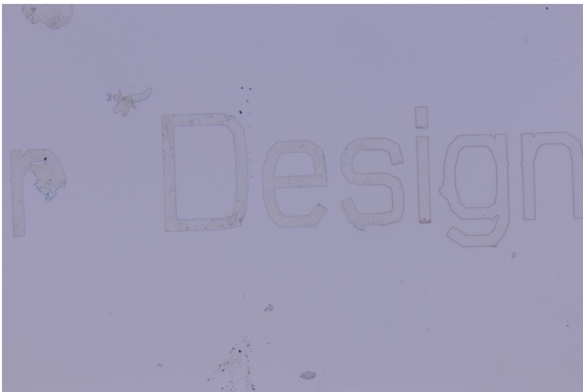
Figure 3.12: Optical microscope image post KOH etch calibration on a (100) test silicon wafer for 30 min. Alignment marks become clearly visible under the optical microscope, allowing subsequent patterns to be aligned.
