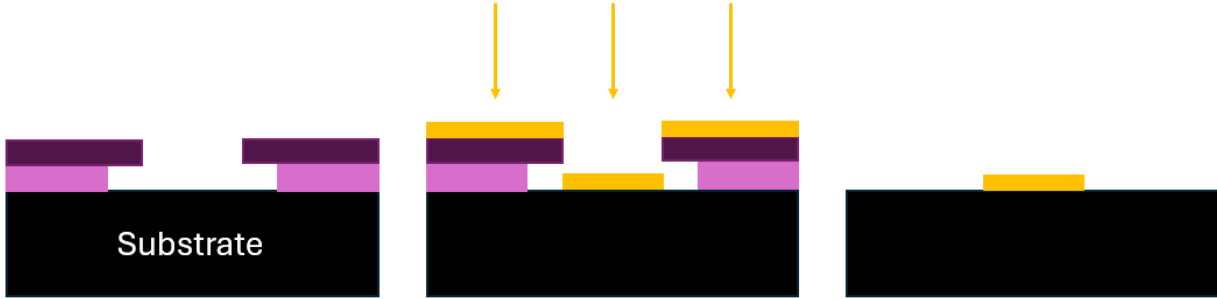
Figure 2.12: Lift off process. A lift-off resist and photoresist bilayer are used to pattern an anisotropic deposition process. The undercut separates masked and unmasked areas.
