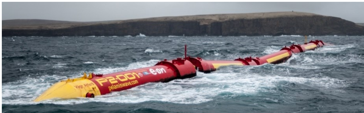
Figure 2.3 – Pelamis wave power converter, now decommissioned [EMEC]
